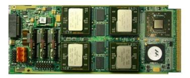
The AMC leverages Serial RapidIO interconnect technology, using IDT's Tsi578 switch to cluster four Freescale MSC8144 multi-core DSPs in an AMC single-width form factor enabling the development of AdvancedTCA and MicroTCA-based systems.
