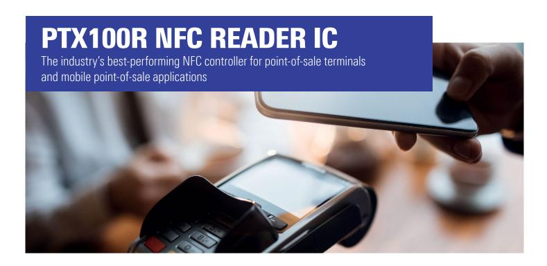
The PTX100R is a comprehensive NFC reader system-on-chip for use in point-of-sale (PoS) terminals and mobile PoS applications. It provides a complete NFC reader implementation optimized for use in contactless payment terminals, including the RF physical layer, power management circuit, and on-chip EMVCo hardware accelerator.
