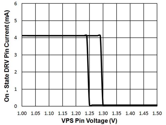
Figure 7.2 : On-State DRV Pin Sink Current (V<sub>DRV</sub>=3.5V) vs. VPS Pin Voltage
