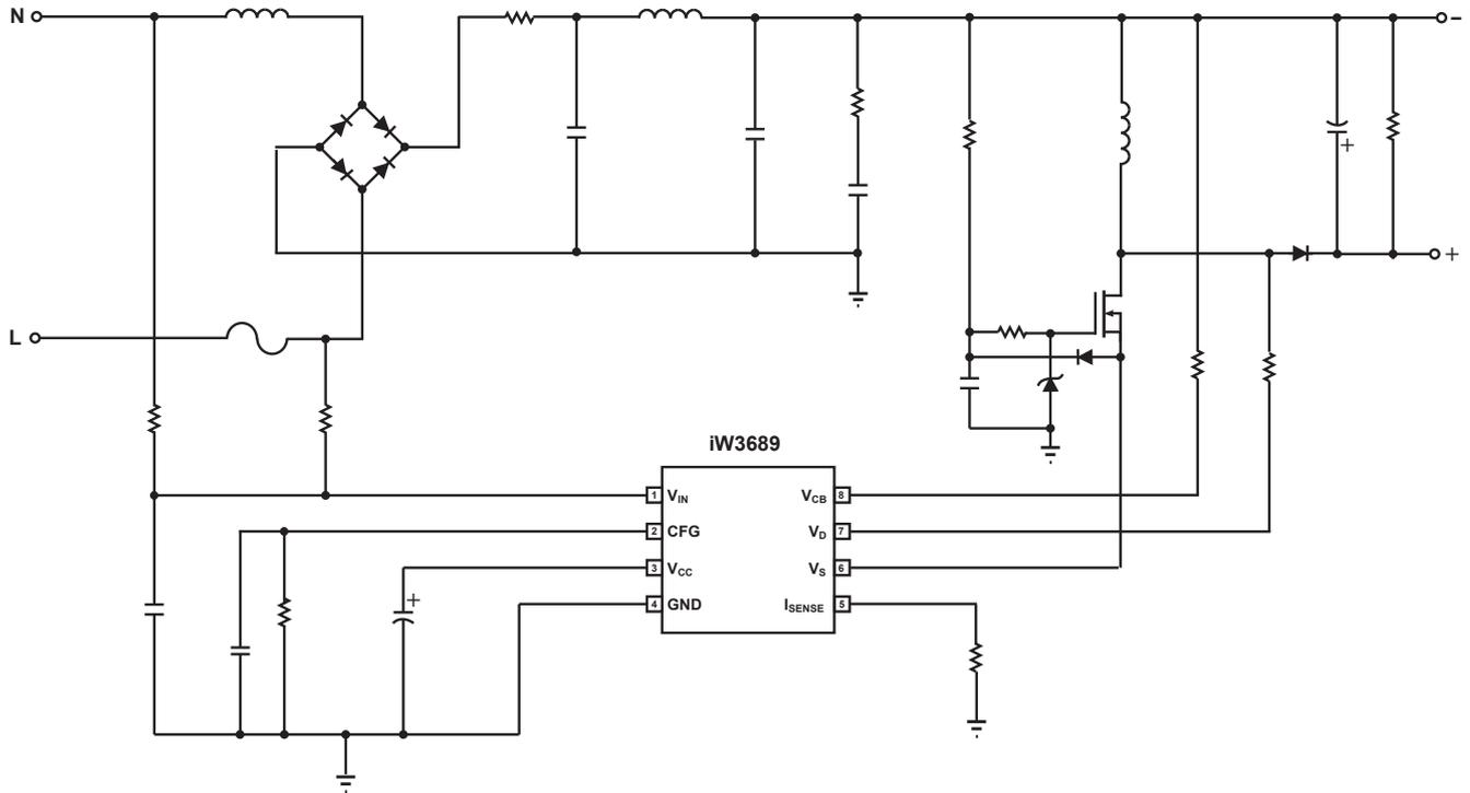
Figure 3.1 : iW3689 Typical Application Circuit
