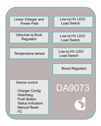
Battery protection features are available to prevent the battery from over-heating and over-discharge. The input is 22 V tolerant and is immune to plug-in of the wrong adaptor. Dynamic power path management enables charging from multiple power sources, and automatically balances current delivered to the system and for charging the battery.
