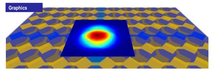
Sensitivity of a mutual capacitance touch surface as simulated in CapExt
