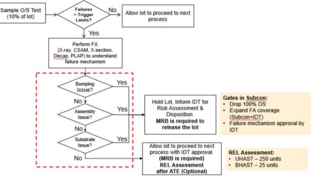
Bumping Issue: Missing bumps, Open bumps, UBM Defects, RDL defects. Assembly Issue: Bump bridge, Missing bump, Delamination, Die Crack. Substrate Issue: Shorting Trace, Open Trace, Open Via.
