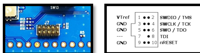
Figure 59: JTAG Pin Connection
