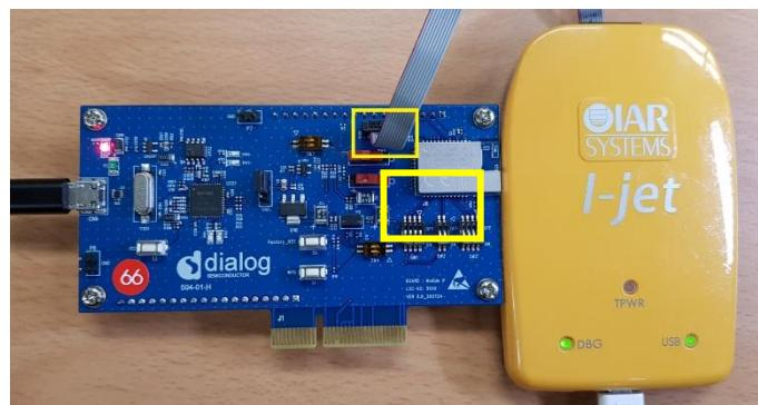
**Figure 27: Connect I-Jet Debugger to the DA16200 (DA16600) EVB**
