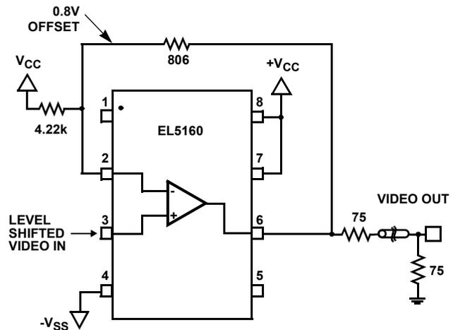
FIGURE 4. DC-RESTORE WITH NEGATIVE SYNC TIP OUTPUT
