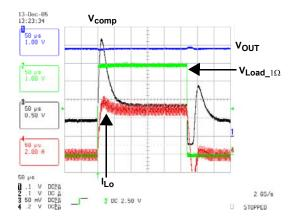
FIGURE 3. TRANSIENT RESPONSE AT 15V VIN
