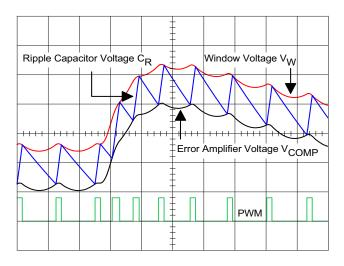
FIGURE 1. MODULATOR LOAD TRANSIENT WAVEFORMS
