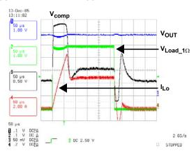
FIGURE 2. TRANSIENT RESPONSE AT 7V VIN
