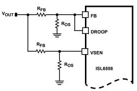
FIGURE 1. VSEN RESISTOR DIVIDER CONFIGURATION
