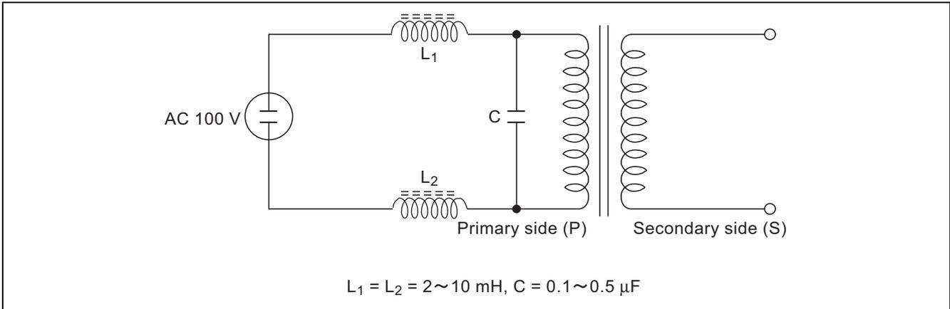
Figure 1 Example Surge Absorber Circuit
