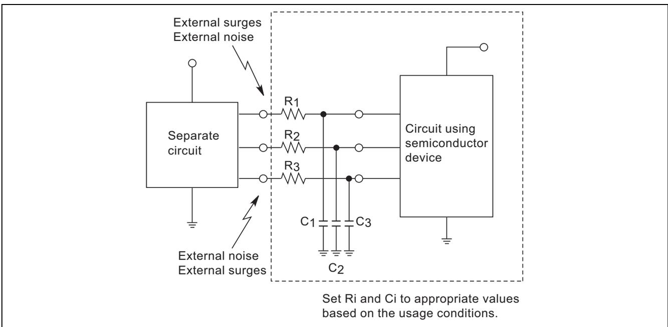
Figure 2 Example Surge Protection Circuit
