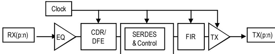
The RX receiver stage of IDT Retimers feature a sensitive analog front end (AFE) and CTLE equalizer for linear distortion (similar to a Repeater's), which is followed by a CDR and DFE stage. The CDR converts the input into the digital domain allowing for packet snooping, sophisticated analysis, and enhanced features such as an on-die scope. The DFE function enables correction of non-linear input signal distortion.
