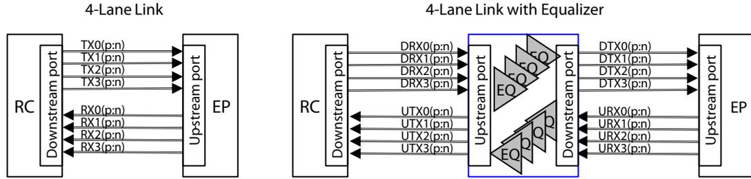
**Port** A group of Transmitters and Receivers located on the same component that operate together. Two ports form the ends of a serial communications link. A four-port Retimer that supports two independent links, each with 4 lanes, is diagrammed below.
