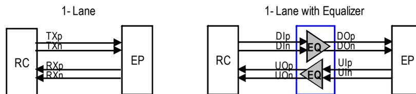
**Link** The collection of two ports and their interconnecting lanes. A link is dual-simplex communications path between two components. A 4-lane link is displayed below.
