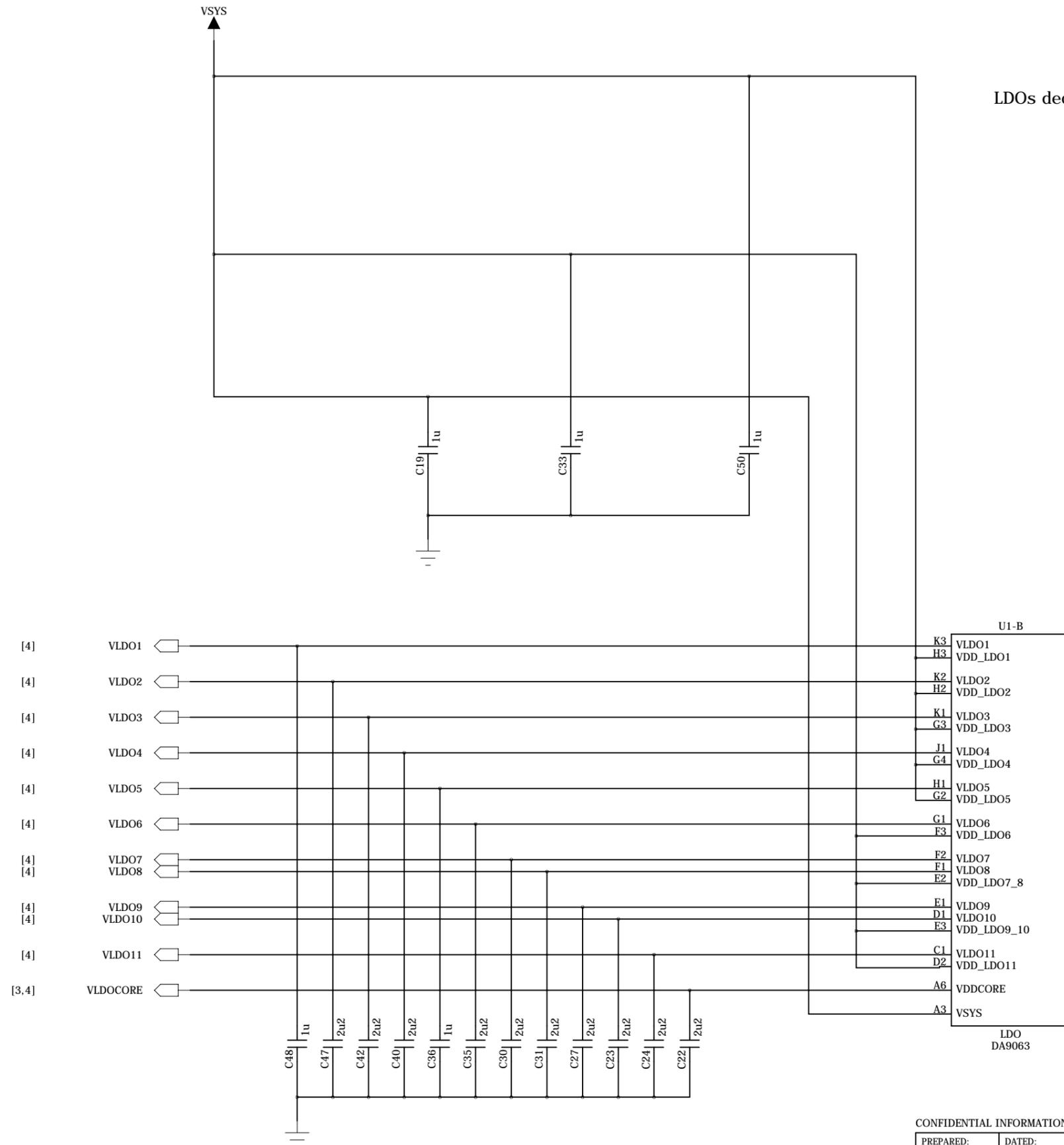
LDOs decoupling: place one capacitor close to each pad group as below:
