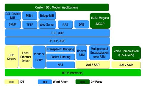
In addition to the Wind River software (shown in blue), the strong 3<sup>rd</sup> party program developed by Wind River will ensure a broad range of additional software modules can be quickly integrated and validated on a RC32355-based platform.
