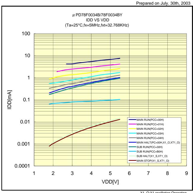
X1\_O:X1 oscillation Operating X1\_S:X1 oscillation Stop XT1\_O:XT1 oscillation Operating
