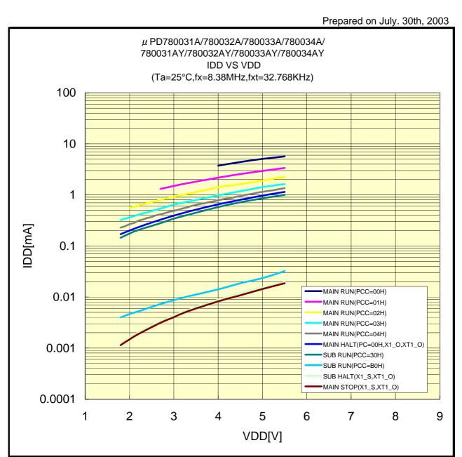
X1\_O:X1 oscillation Operating X1\_S:X1 oscillation Stop
