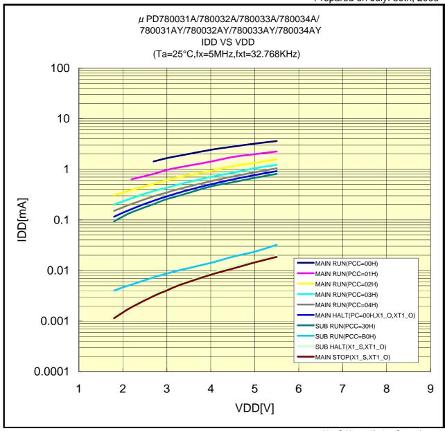
X1\_O:X1 oscillation Operating X1\_S:X1 oscillation Stop XT1\_O:XT1 oscillation Operating
