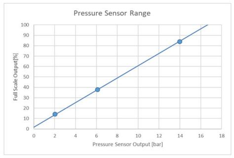
Figure 3. Assignment Input Resistive Range to SSC-output
