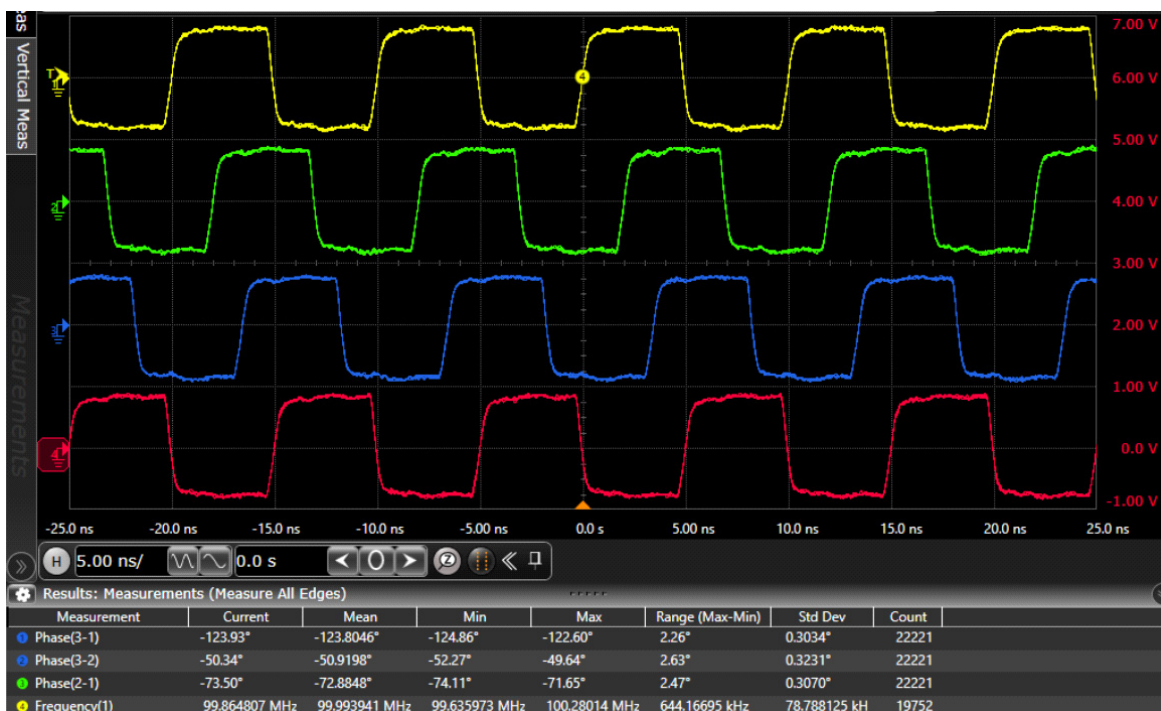
Figure 10. Bench Measurement of OUT2 (120° of Skew) vs OUT1 (60° of Skew), Phase (2–1)
