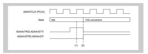
Figure 22-9 Software start trigger timing example
