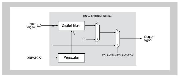
Figure 2-7 Digital filter type D block diagram
