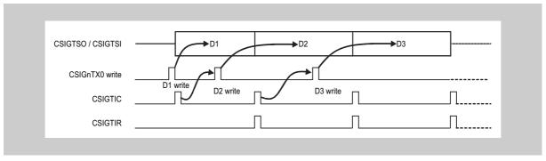
**Figure 19-15** Generation of CSIGTIC at the beginning of communication
