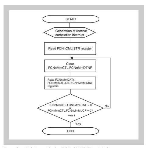
Figure 18-34 Reception via interrupt (using FCNnCMLISTR register)
