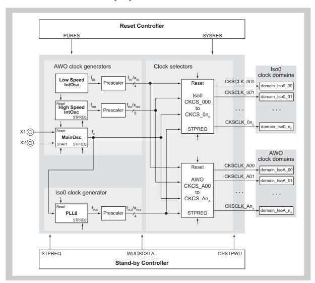
Figure 7-2 Clock Controller structure
