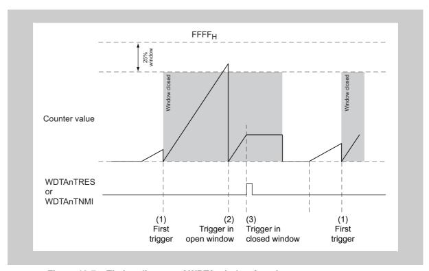
Figure 13-7 Timing diagram of WDTA window function
