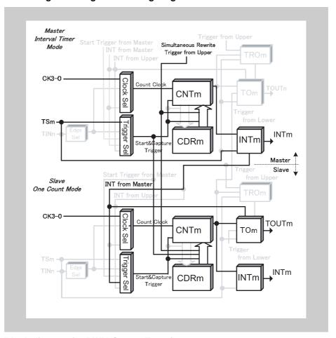
Figure 15-51 Block diagram for PWM Output Function
