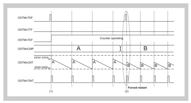
Figure 12-6 Timing diagram of forced restart in interval timer mode
