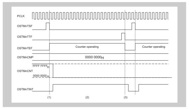
Figure 12-7 Timing diagram when OSTMnCMP = 0000 0000<sub>H</sub> in interval timer mode
