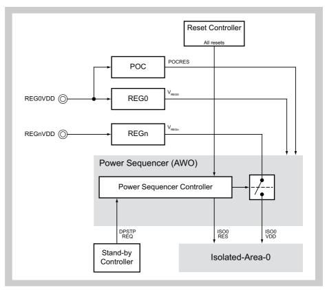
Figure 24-5 Power supply control scheme
