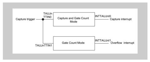
Figure 15-17 Combination of Capture and Gate Count Mode and Gate Count Mode
