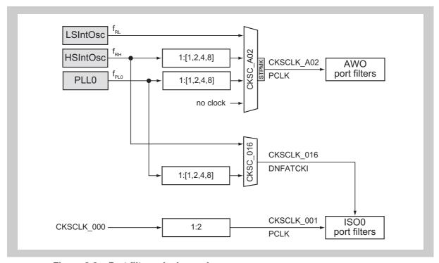
Figure 2-2 Port filters clock supply
