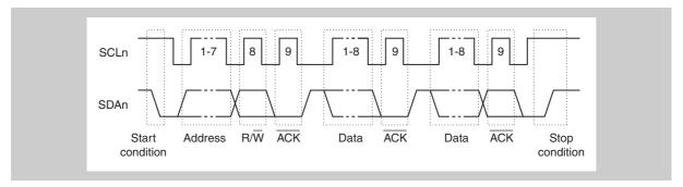
Figure 20-4 I<sup>2</sup>C bus serial data transfer timing
