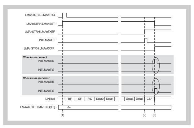
Figure 17-7 LIN frame transmission in LIN master mode
