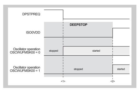
Figure 8-3 OSCWUFMSK effect on MainOsc start time
