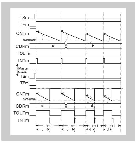
Figure 15-52 General timing diagram for PWM Output Function
