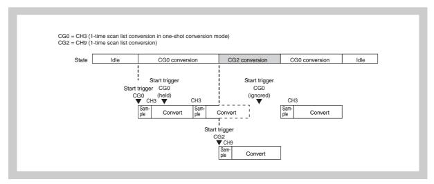
Figure 22-7 Start Trigger for a different CG before end of conversion (ADAAnCTL1.ADAAnTRM0 = 0)
