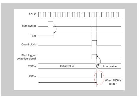
Figure 14-13 Start timing of Interval Timer Mode, Judge Mode, Capture Mode, Up
