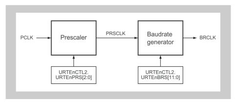
Figure 16-17 Configuration of baud rate generator
