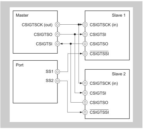
Figure 19-6 Master to multiple slaves connection
