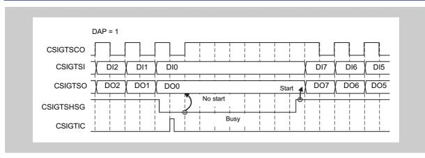
Figure 19-20 Master's reaction to CSIGTSHSG (CSIGnCFG0.CSIGnDAP = 1)
