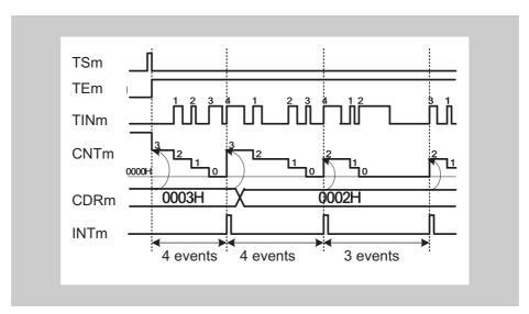
Figure 14-57 General timing diagram for External Event Count Function
