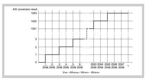
Figure 22-16 Conversion characteristics of 10-bit A/D converter (ADAAnCTL1.ADAAnCTYP = 1)
