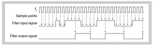
Figure 2-6 Digital filter function
