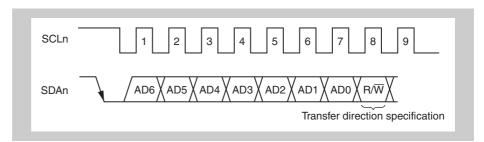
Figure 20-7 Transfer direction specification
