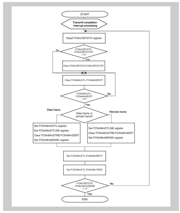
Figure 18-25 Transmission via interrupt (using FCNnCMTGTX register)
