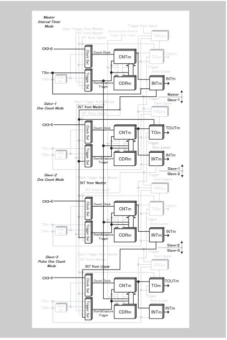
Figure 14-74 Block diagram for Delay Pulse Output Function
