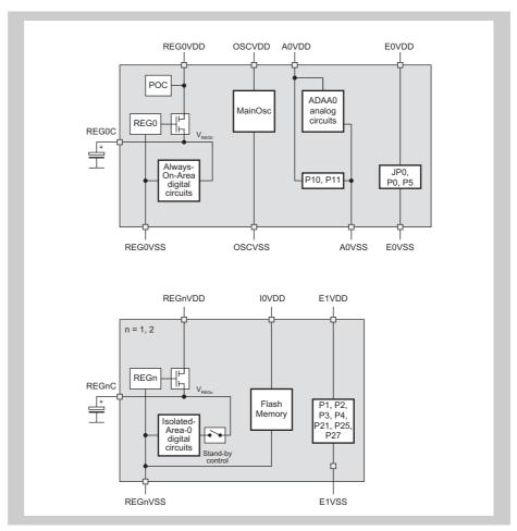
Figure 24-4 V850E2S/FJ4-L power supply scheme
