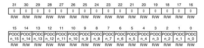
**Note** The control bits of the JTAG port register JPODC0 are named JPODC0\_[31:0].
