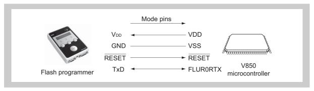
Figure 6-2 Communication with flash programmer via FLUR0
