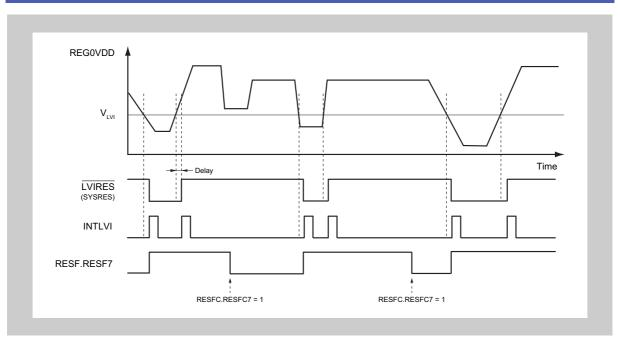
Figure 11-3 LVI reset and interrupt timing
