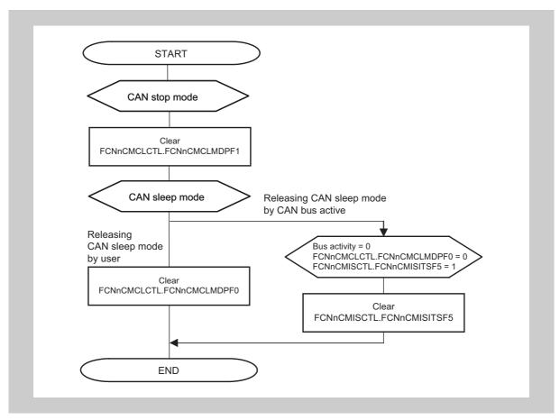
Figure 18-39 Clear CAN Controller sleep/stop mode
