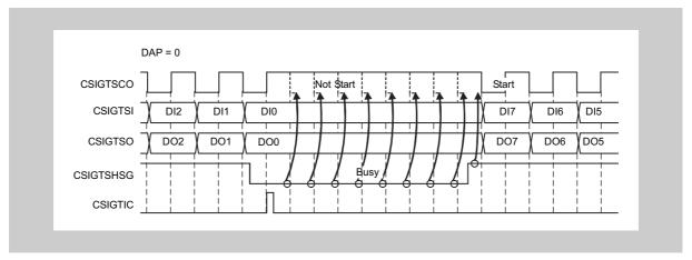
Figure 19-19 Master's reaction to CSIGTSHSG (CSIGnCFG0.CSIGnDAP = 0)
