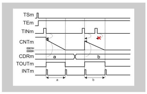
Figure 14-30 General timing diagram for One-Pulse Output Function
