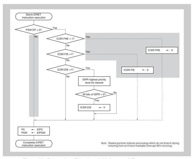
Figure 4-5 Restore from El level maskable interrupt INTn
