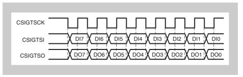
Figure 19-3 Transmit/receive in master mode
