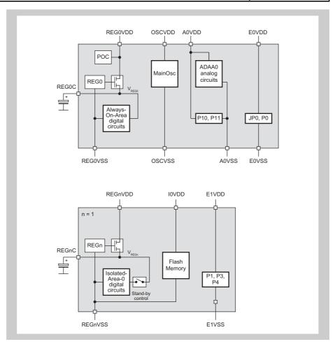
Figure 24-3 V850E2S/FG4-L power supply scheme
