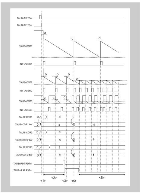
Figure 14-9 Simultaneous rewrite when INTTAUBnIm is generated on an upper channel specified by TAUBnRDC.RDCm
