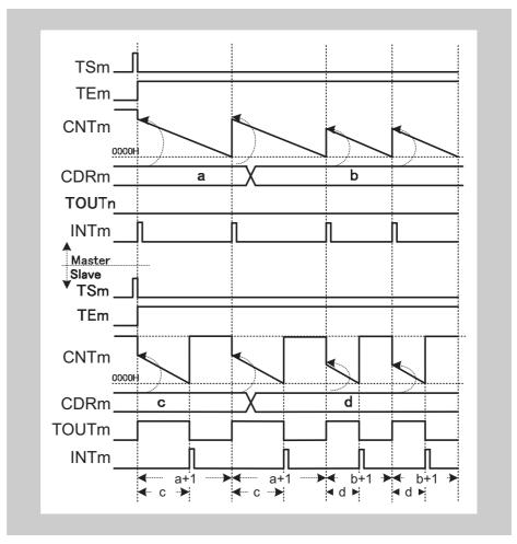
Figure 14-70 General timing diagram for PWM Output Function
