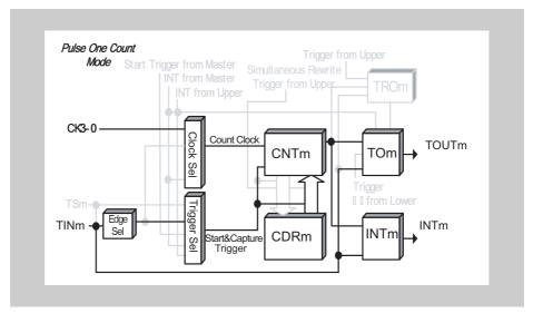
Figure 14-29 Block diagram for One-Pulse Output Function
