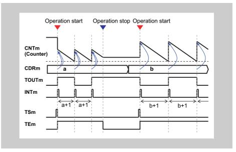
Figure 14-23 Operation stop and restart, TAUBnCMORm.MD0 = 1
