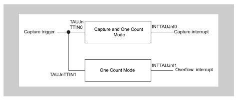
Figure 15-13 Combination of Capture and One Count Mode and One Count Mode
