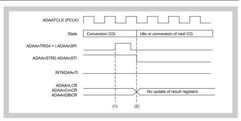
Stop trigger timing, if generated before A/D conversion end **Figure 22-11**
