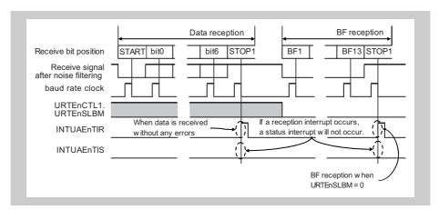
Figure 16-5 Reception interrupt request timing
