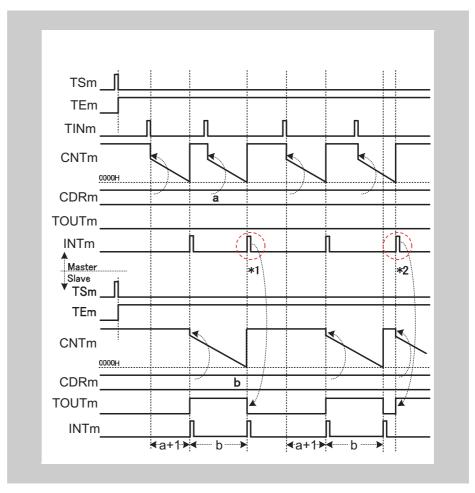
Figure 14-85 Interval of TAUBnTTINm ≤ delay time + pulse width +1
