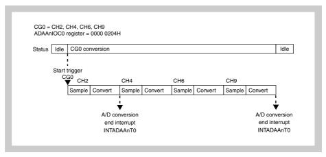
**Figure 22-14** Generation of A/D conversion end interrupt INTADAAnTi
