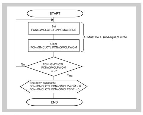
Figure 18-42 Forced shutdown process
