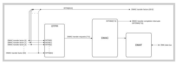
Figure 5-1 DMA trigger and interrupt signals connections
