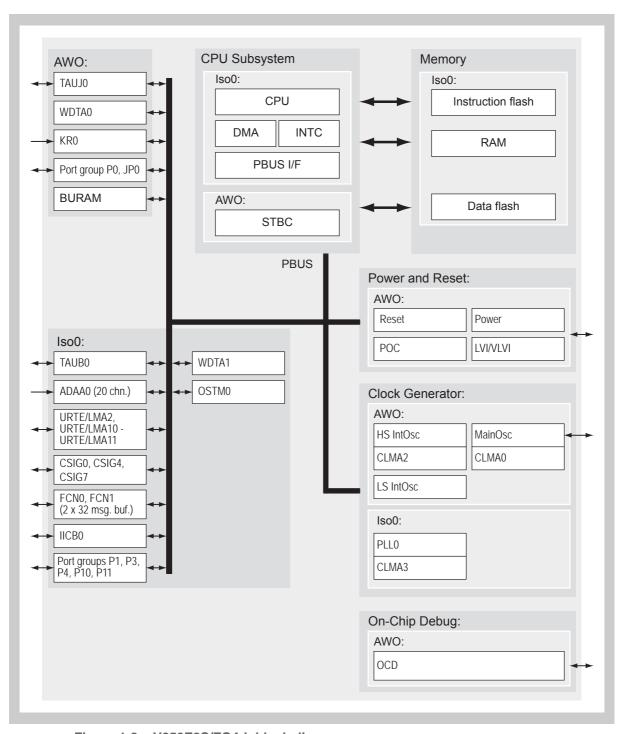
Figure 1-3 V850E2S/FG4-L block diagram
