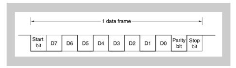
(c) 8-bit data length, MSB first, even parity, 1 stop bit, transfer data: 55<sub>H</sub>, URTEnTTXD inversion
