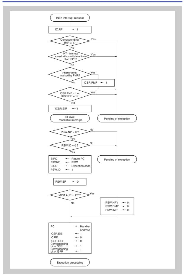
Figure 4-4 Processing upon occurrence of INTn interrupt request
