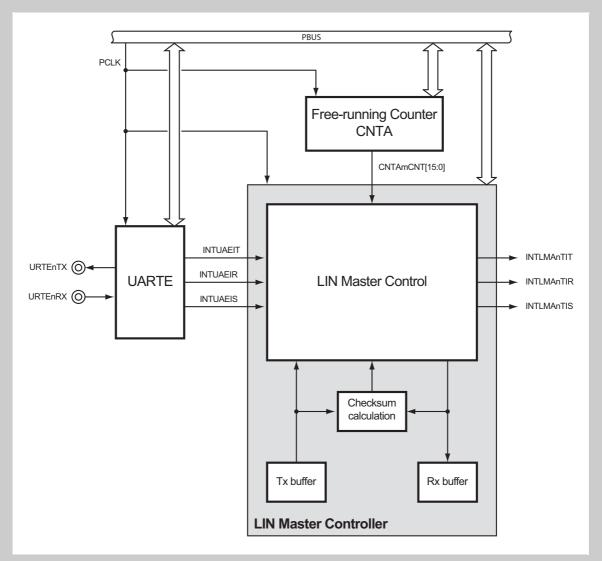
Figure 17-3 LIN Master Controller environment
