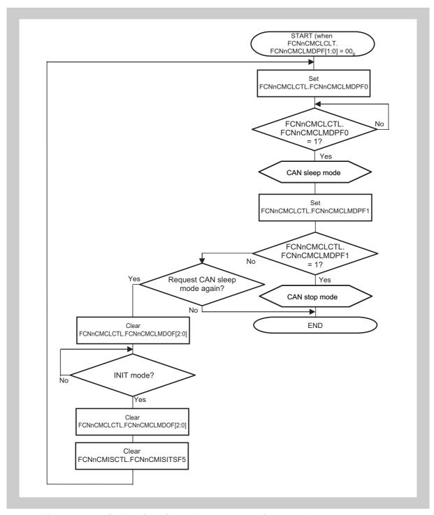
Figure 18-38 Setting CAN Controller sleep mode/stop mode
