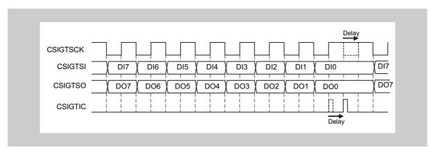
Figure 19-13 Interrupt delay function (CSIGnCTL1.CSIGnSIT = 1)
