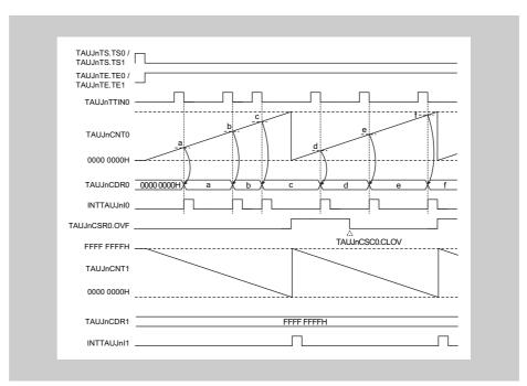
Figure 15-16 Interrupt generation via combination of Count Capture Mode and Interval Timer Mode
