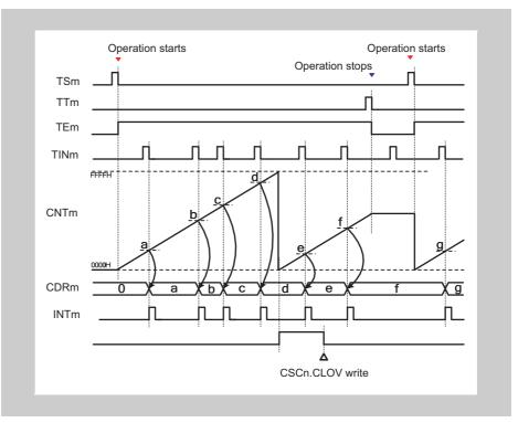
Figure 14-68 Operation stop and restart, TAUBnCMORm.MD0 = 0, TAUBnCMURm.TIS[1:0] = 00
