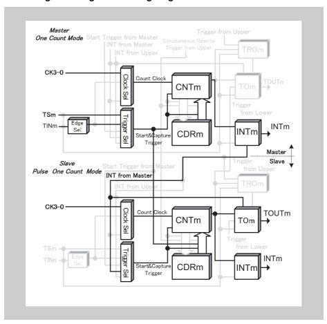
**Figure 14-80** Block diagram for One-Shot Pulse Output Function
