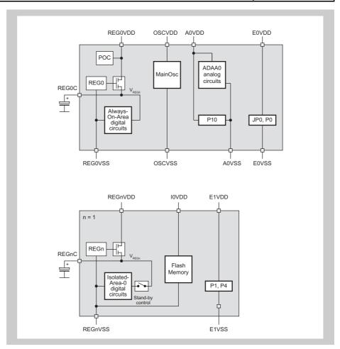
Figure 24-1 V850E2S/FE4-L power supply scheme
