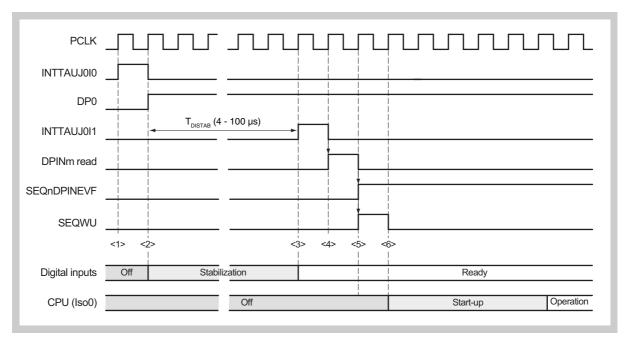
Wake-up Sequencer operation in digital input mode - DPINm change Figure 9-6
