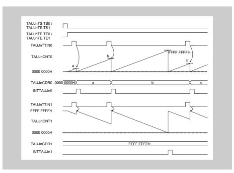
Figure 15-12 Interrupt generation via combination of Capture Mode and Interval Timer Mode
