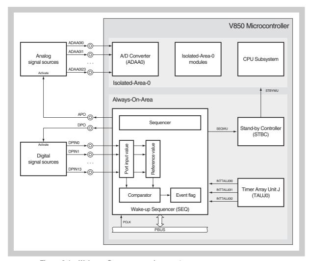
Figure 9-1 Wake-up Sequencer environment
