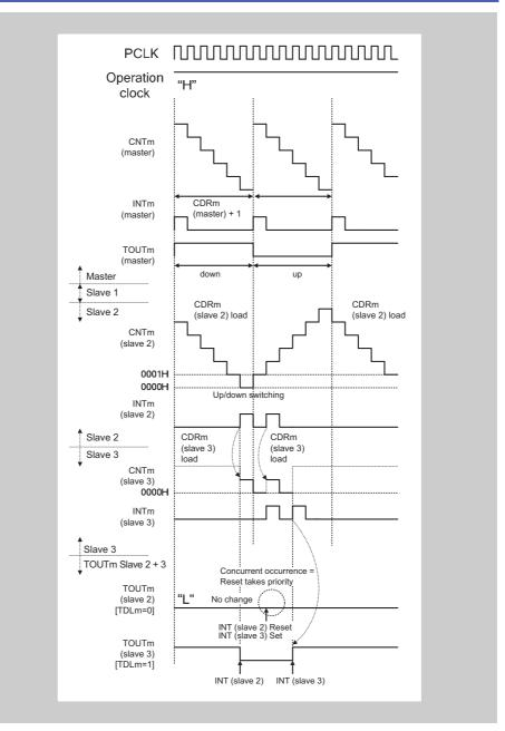
Figure 14-96 TAUBnCDRm (master) =  $0005_{H}$ , TAUBnCDRm (slave 2) =  $0005_{H}$ , TAUBnCDRm (slave 3) =  $0001_{H}$  PWM signal width (positive phase) = 0
