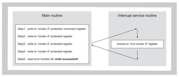
Figure 3-16 Successful register protection unlock sequence
