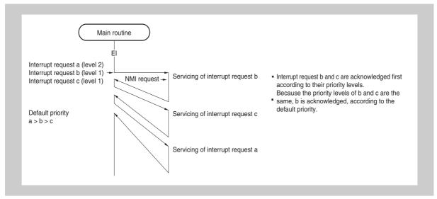
Figure 4-8 Example of servicing simultaneously generated interrupt requests
