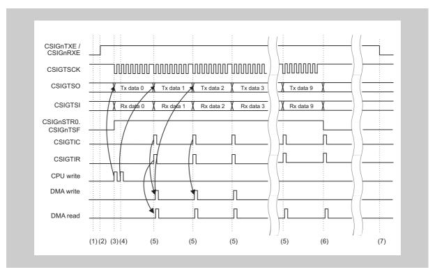
Figure 19-27 Communication in master mode
