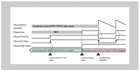
Figure 15-6 General procedure for specifying a TAUJnTTOUTm channel output mode
