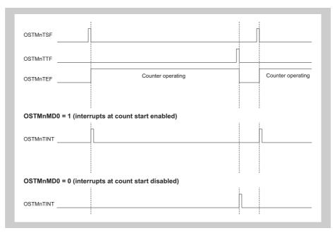
Figure 12-4 Interrupt generation at count start
