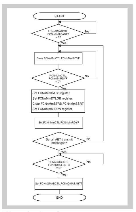
Figure 18-23 ABT message transmit processing
