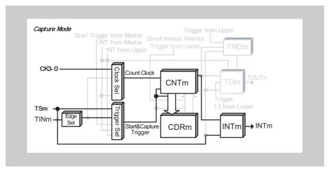
Figure 14-31 Block diagram for TAUBnTTINm Input Pulse Interval Measurement Function
