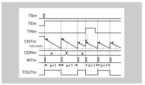
Figure 15-28 Counter triggered by rising TAUJnTTINm input edge (TAUJnCMURm.TIS[1:0] = 01<sub>B</sub>), TAUJnCMORm.MD0 = 1
