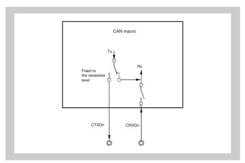
Figure 18-13 CAN Controller terminal connection in self-test mode
