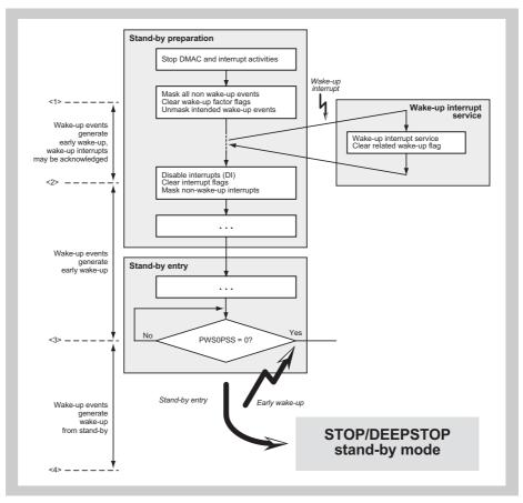
Figure 8-8 Saving wake-up events during stand-by preparation
