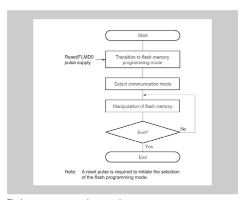
Figure 6-4 Flash memory programming procedure
