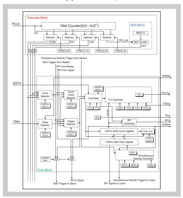
Figure 15-2 Block diagram of the TAUJ
