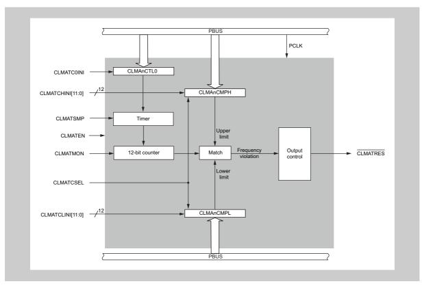
Figure 7-15 Block diagram of the Clock Monitor A
