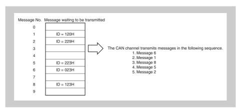
Figure 18-10 Message processing example
