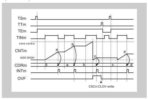
Figure 15-45 Operation stop and restart, TAUJnCMURm.TIS[1:0] = 11<sub>B</sub>
