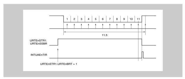
Figure 16-9 Normal BF reception (stop bit after more than 10.5 "L" bits)
