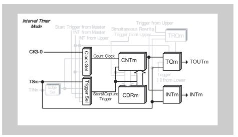
Figure 14-19 Block diagram for Interval Timer Function
