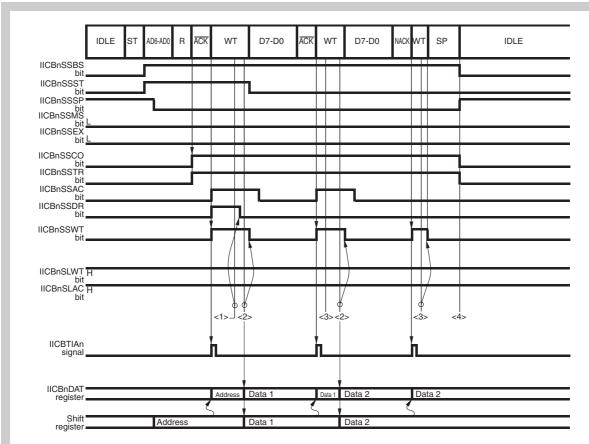
**Note** During data transmission, set the IICBnCTL0.IICBnSLWT bit (to 1) so that the IICBn enters the wait state at the falling edge of the 9th clock.
