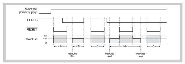
Figure 11-6 MainOsc behaviour during RESET
