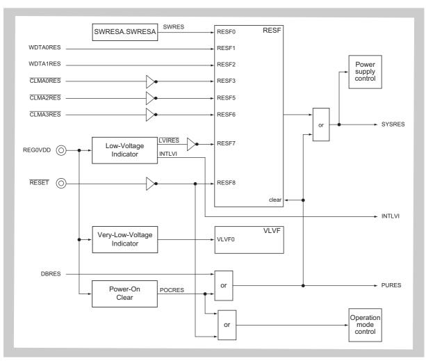
Figure 11-1 Block diagram of the Reset Controller
