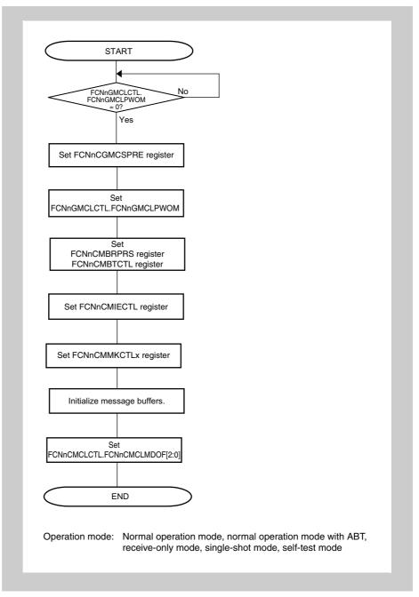
Figure 18-18 Re-initialization with Software Reset function
