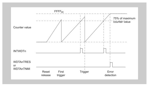
Figure 13-6 Timing diagram of WDTA 75% interrupt output
