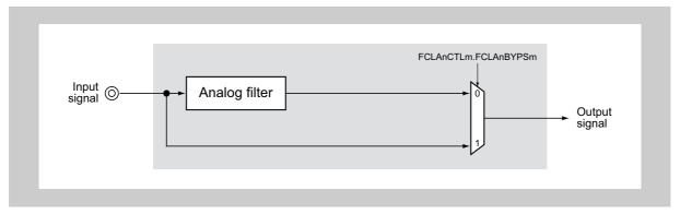
Figure 2-4 Analog filter type B block diagram
