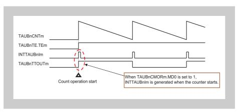
Figure 14-16 INTTAUBnIm generated when counter starts
