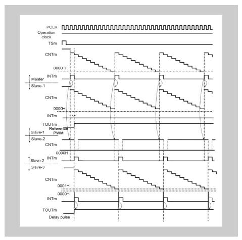
If the value of TAUBnCDRm (slave 1 and 3) is higher than the value of TAUBnCDRm (master), the counter of the slave channels cannot reach 0000<sub>H</sub> and cannot generate interrupts. TAUBnTTOUTm of channels 1 and 3 remain in the active state.
