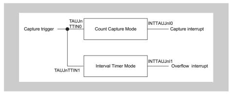
Figure 15-15 Combination of Count Capture Mode and Interval Timer Mode
