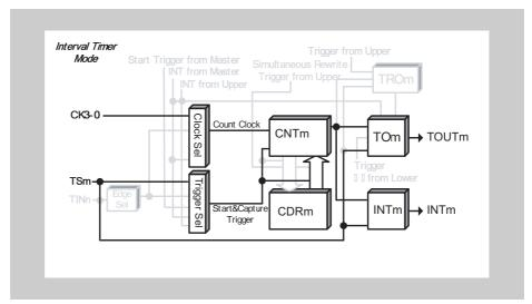
Figure 15-20 Block diagram for Interval Timer Function
