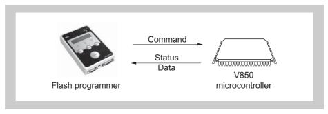
Figure 6-9 Communication commands exchange
