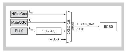
Figure 20-1 IICB clock supply
