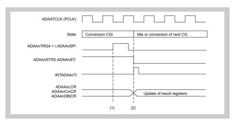
Figure 22-12 Stop trigger timing, if generated after A/D conversion end
