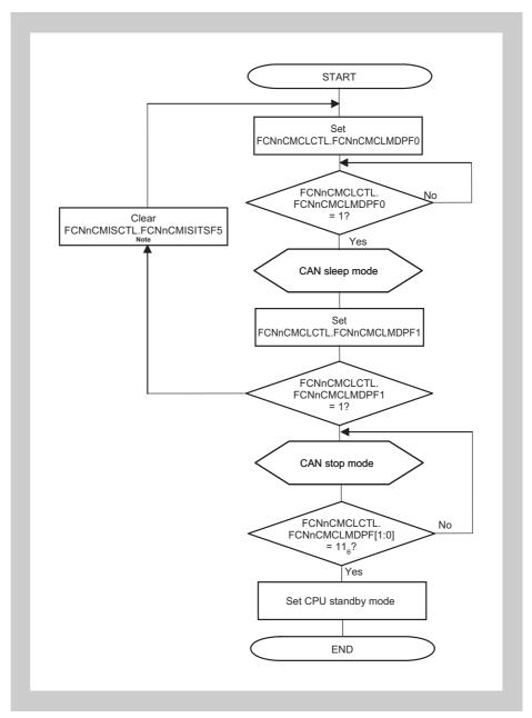
Setting CPU stand-by (from CAN Controller stop mode) Figure 18-45
