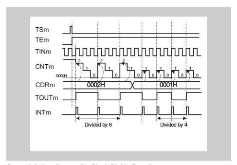
Figure 14-62 General timing diagram for Clock Divide Function
