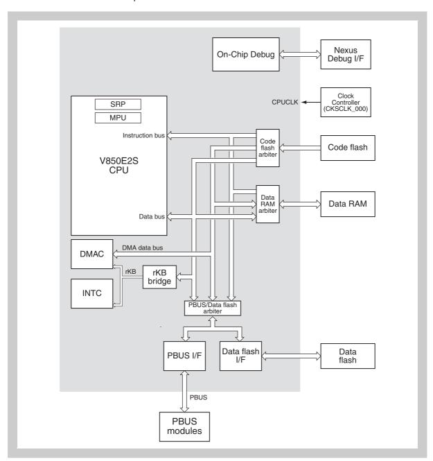
Figure 3-5 CPU Subsystem
