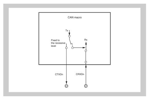
Figure 18-12 CAN Controller terminal connection in receive-only mode
