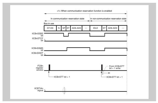
Figure 20-12 Valid times to write to IICBnDAT register
