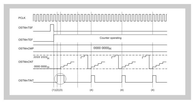
Figure 12-9 Timing diagram when OSTMnCMP = 0000 0000<sub>H</sub> in free-run compare mode
