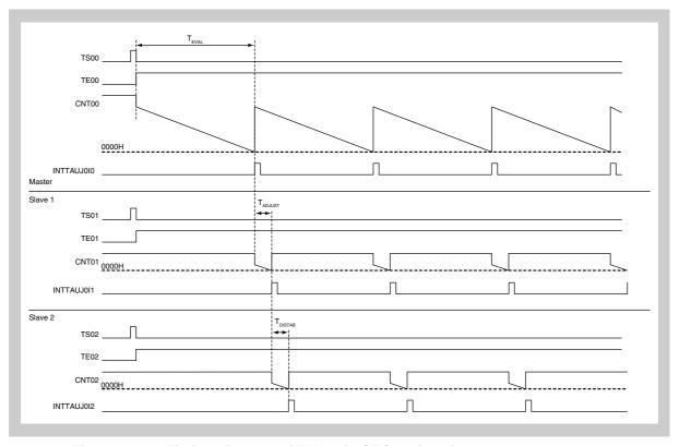
Figure 9-11 Timing diagram of TAUJ0 in SEQn mixed input mode
