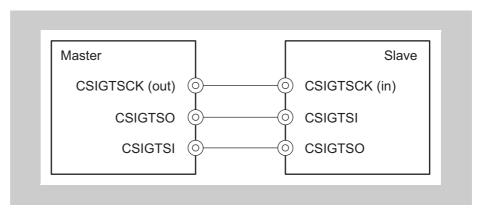
Figure 19-5 Simple master/slave connection
