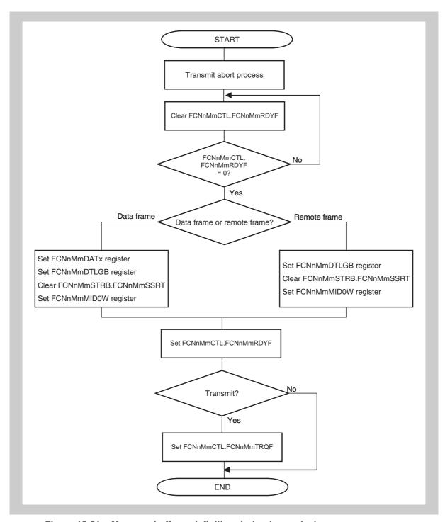
Figure 18-21 Message buffer redefinition during transmission
