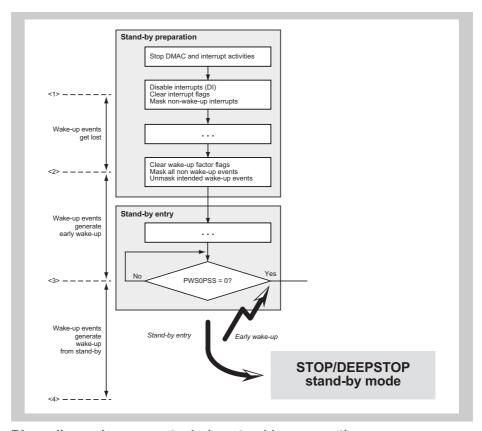
Figure 8-7 Discarding wake-up events during stand-by preparation
