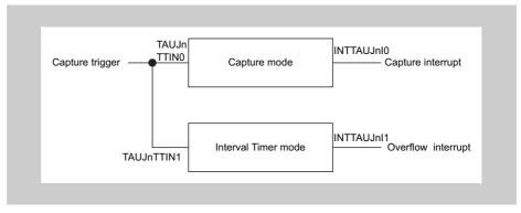
Figure 15-11 Combination of Capture Mode and Interval Timer Mode
