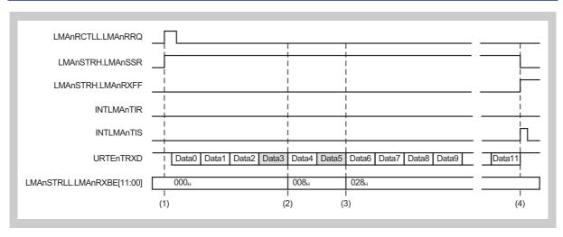
Figure 17-6 Data reception in UART buffer mode with UART reception errors
