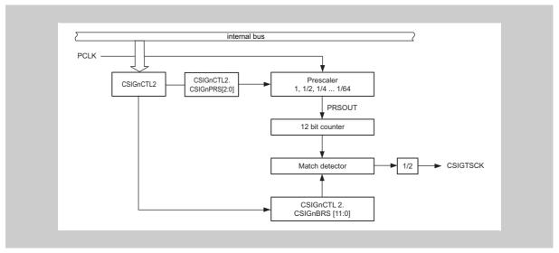
Figure 19-7 BRG block diagram
