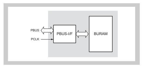
Figure 3-13 Block diagram of the Back-up RAM
