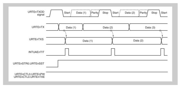
Figure 16-14 Continuous transmission operation timing - transmission start
