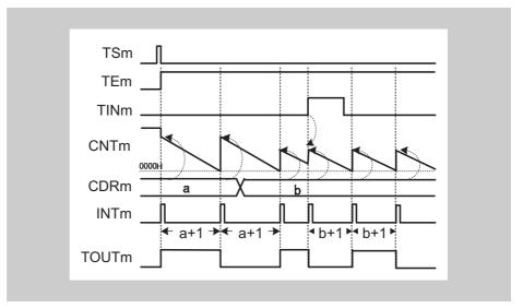
Figure 14-28 Counter triggered by rising TAUBnTTINm input edge (TAUBnCMURm.TIS[1:0] = 01<sub>B</sub>), TAUBnCMORm.MD0 = 1
