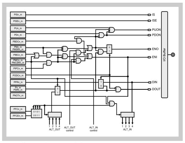
Figure 2-1 Port control logic diagram
