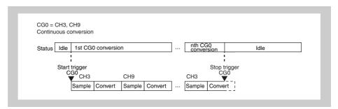
Figure 22-8 Continuous conversion mode
