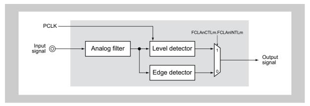
Figure 2-3 Analog filter type A block diagram
