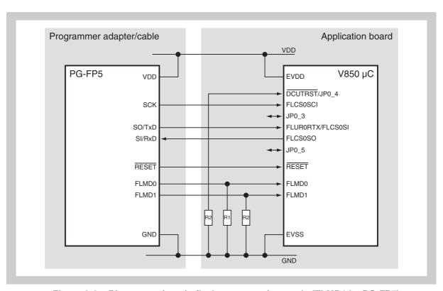
Figure 3-8 Pin connections in flash programming mode (FLMD1 by PG-FP5)
