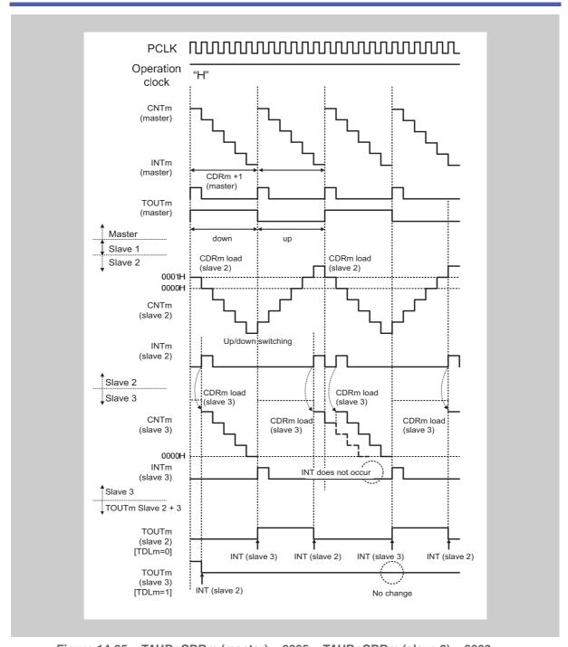
Figure 14-95 TAUBnCDRm (master) =  $0005_{\rm H}$ , TAUBnCDRm (slave 2) =  $0002_{\rm H}$ , TAUBnCDRm (slave 3) =  $0004_{\rm H}$ PWM signal width (negative phase)  $\geq$  Carrier cycle
