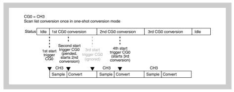
Figure 22-6 Start Trigger for the same CG before end of conversion
