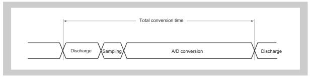
Figure 22-18 Timing when discharge function is enabled
