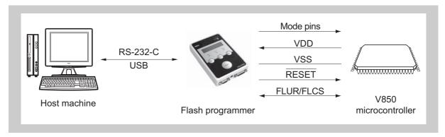
Figure 6-1 Environment to write program to flash memory
