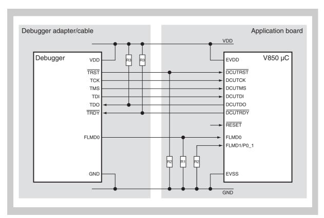
Figure 3-7 Pin connections in debug mode
