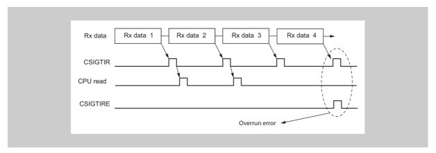
Figure 19-26 Overrun error detection - example
