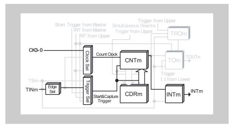
Figure 14-48 Block diagram for Overflow Interrupt Output Function (During TAUBnTTINm Input Period Count Detection)
