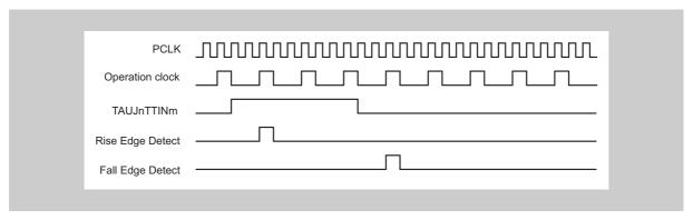
Figure 15-19 Basic edge detection timing
