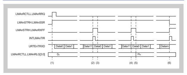
Figure 17-5 Data reception in UART buffer mode
