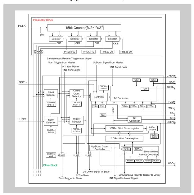
Figure 14-4 Block diagram of the TAUB
