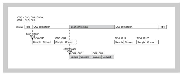
Figure 22-3 Immediate interruption of A/D conversion of CG0 (ADAAnCTL1.ADAAnTRM0 = 0)
