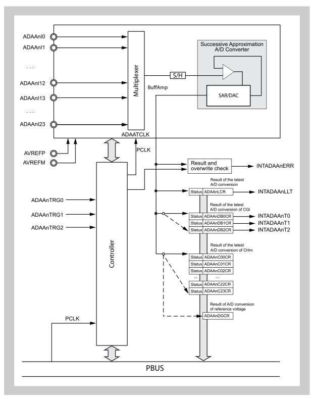
Figure 22-2 Block diagram of the ADAA
