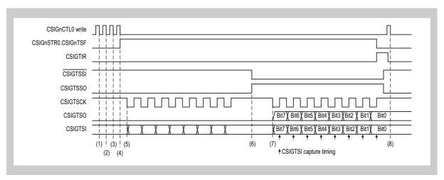
Figure 19-12 Rx/Tx communication timing in slave mode
