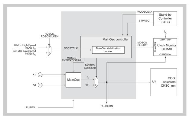
Figure 7-4 Main Oscillator clock generator
