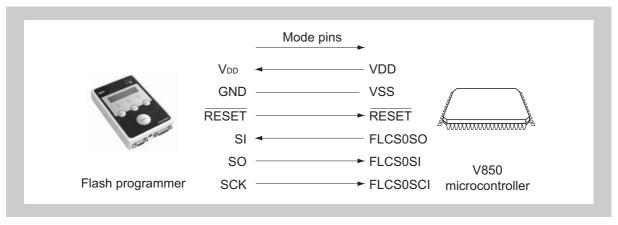
Figure 6-3 Communication with flash programmer via FLCS0
