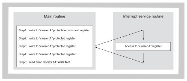
Figure 3-15 Disruption of register protection unlock sequence
