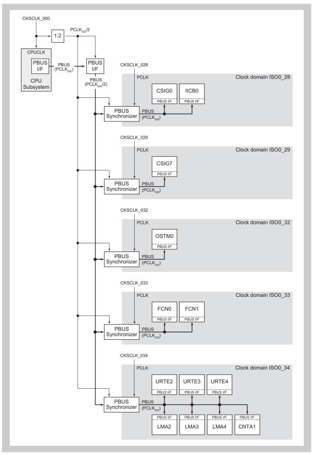
Figure 7-13 Clock domains ISO0\_28, ISO0\_29, ISO0\_32 to ISO0\_34
