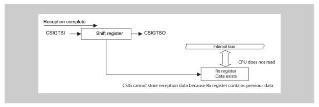
Figure 19-25 Overrun error detection
