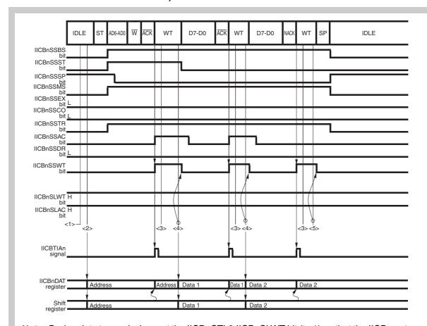
**Note** During data transmission, set the IICBnCTL0.IICBnSLWT bit (to 1) so that the IICBn enters the wait state at the falling edge of the 9th clock.
