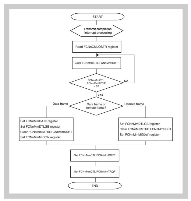
**Figure 18-24** Transmission via interrupt (using FCNnCMLOSTR register)
