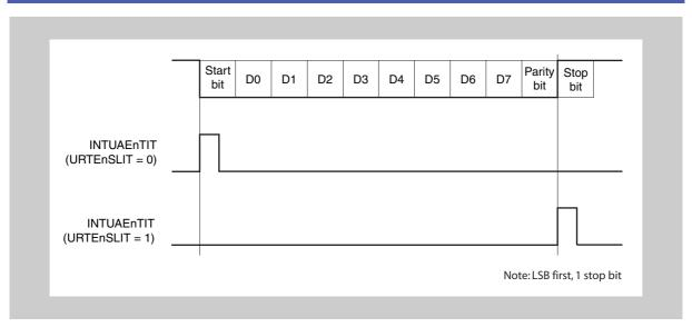
Figure 16-12 Transmission interrupt timing
