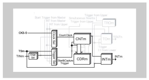
Figure 15-48 Block diagram for TAUJnTTINm Input Position Detection Function
