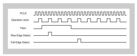
Figure 14-18 Basic edge detection timing
