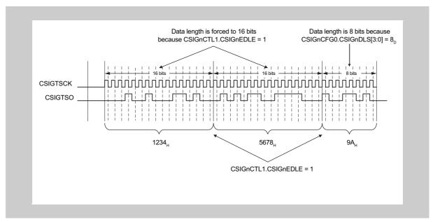
Figure 19-9 EDL timing diagram
