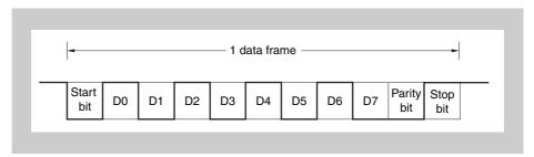
(b) 8-bit data length, MSB first, even parity, 1 stop bit, transfer data: 55<sub>H</sub>
