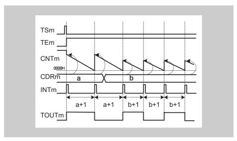
Figure 14-20 General timing diagram for Interval Timer Function
