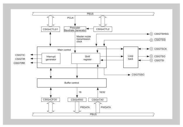
Figure 19-2 CSIG block diagram
