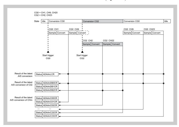
Figure 22-15 Storage of A/D conversion result
