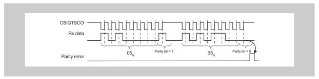
Figure 19-24 Parity check example
