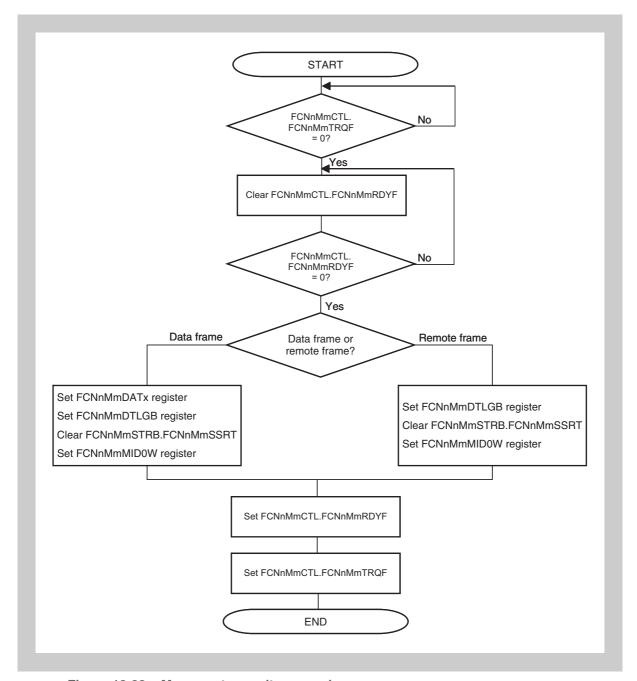
Figure 18-22 Message transmit processing
