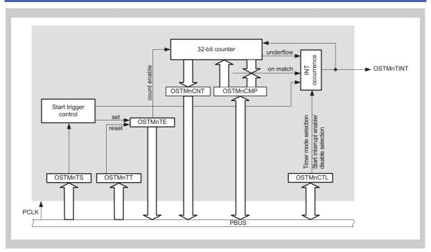
Figure 12-2 Block diagram of the OS Timer
