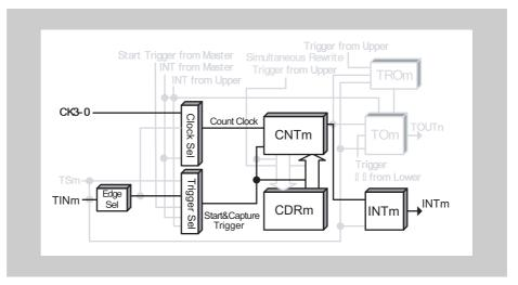
Figure 15-46 Block diagram for Overflow Interrupt Output Function (During TAUJnTTINm Input Period Count Detection)
