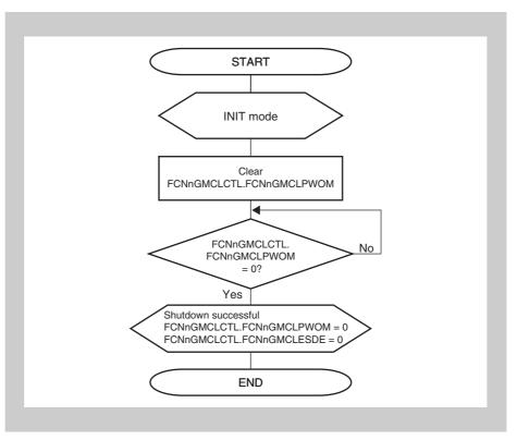
Figure 18-41 Normal shutdown process
