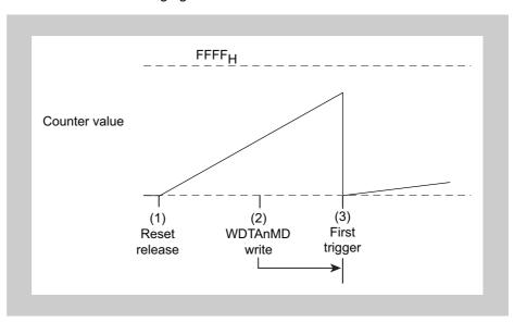
Figure 13-3 Timing diagram of WDTA start in automatic start mode
