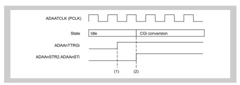
Figure 22-10 Hardware start trigger timing
