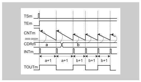
Figure 15-21 General timing diagram for Interval Timer Function
