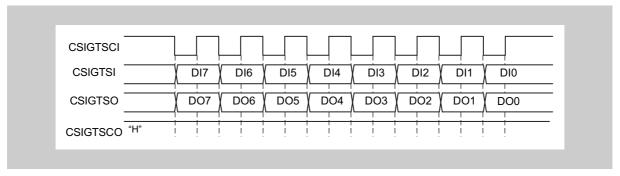
Figure 19-4 Transmit/receive in slave mode
