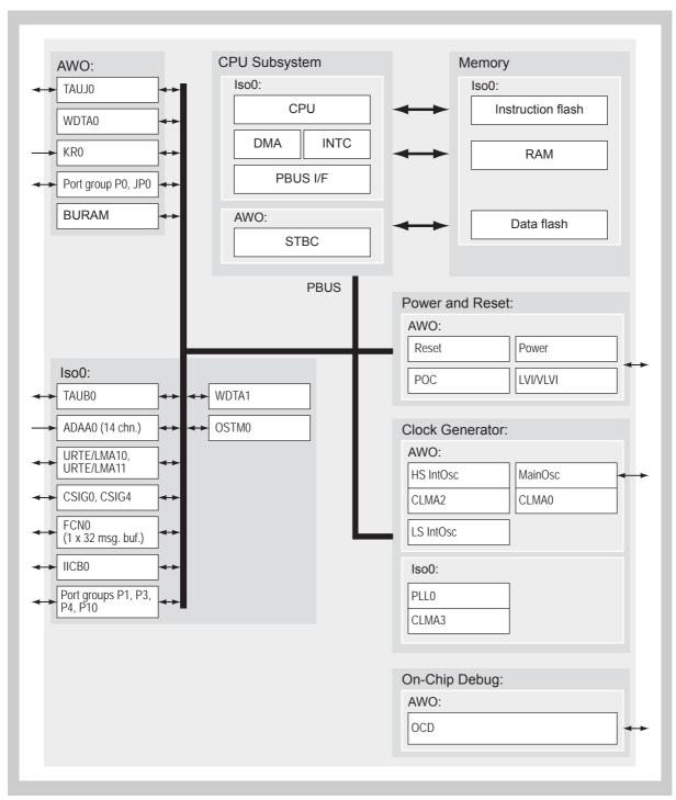
Figure 1-2 V850E2S/FF4-L block diagram
