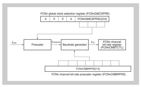
Figure 18-15 CAN Controller clocks
