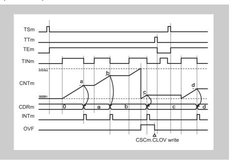
Figure 14-47 Operation stop and restart, TAUBnCMURm.TIS[1:0] = 11<sub>B</sub>
