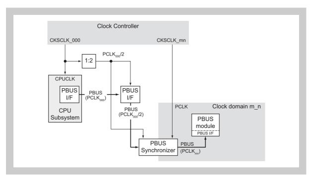
Figure 3-2 PBUS synchronizer
