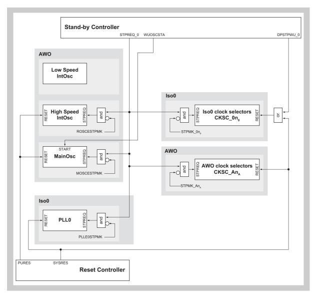
Figure 7-3 Clock Controller stand-by mode and reset signals
