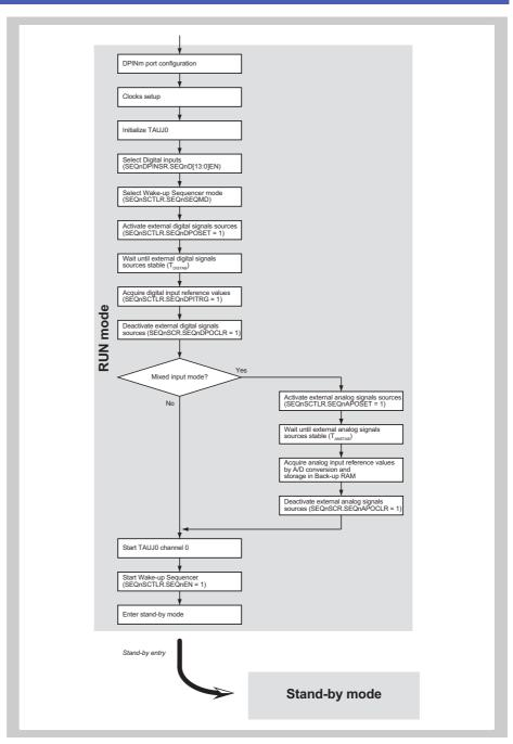
Figure 9-3 Wake-up Sequencer setup
