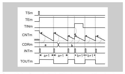
Figure 14-27 General timing diagram for TAUBnTTINm Input Interval Timer Function
