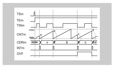
Figure 14-32 General timing diagram for TAUBnTTINm Input Pulse Interval Measurement Function
