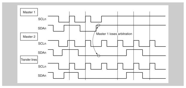
Figure 20-11 Arbitration timing example
