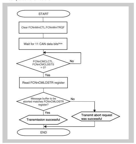
Transmission abort processing (except normal operation mode with **Figure 18-27** ABT)
