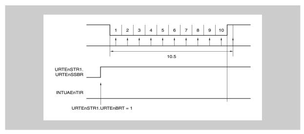
Figure 16-10 BF reception error (stop bit within 10.5 "L" bits)
