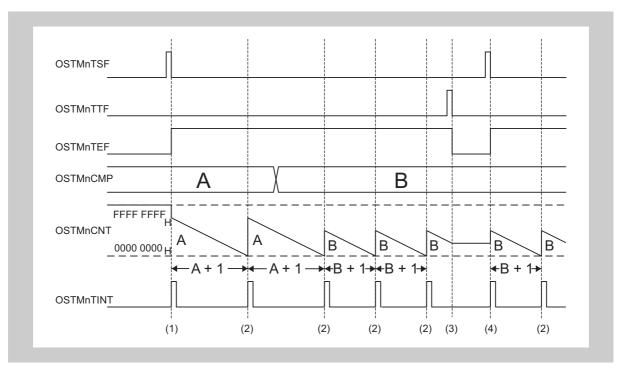
Figure 12-5 Timing diagram of OSTM in interval timer mode
