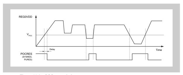
Figure 11-2 POC reset timing
