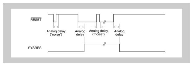
Figure 11-5 External RESET timing
