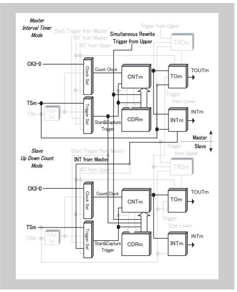
Figure 14-86 Block diagram for Triangle PWM Output Function
