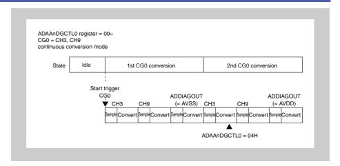
Figure 22-17 ADDIAGOUT change during A/D conversion
