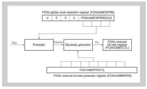
Figure 18-4 CAN Controller clocks
