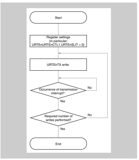
Figure 16-13 Continuous transmission processing flow
