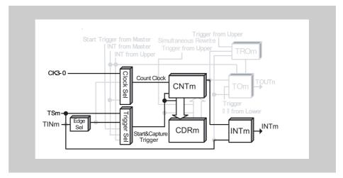
Figure 15-43 Block diagram for TAUJnTTINm Input Period Count Detection Function
