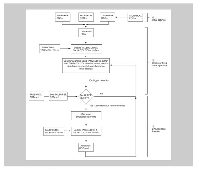
Figure 14-6 General procedure for simultaneous rewrite
