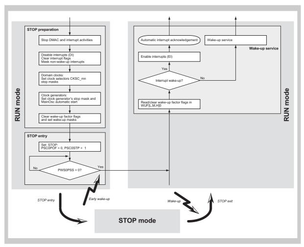
Figure 8-5 Recommended flow of STOP mode
