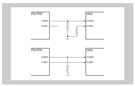
Figure 6-5 Example of connection to flash programmer PG-FP5
