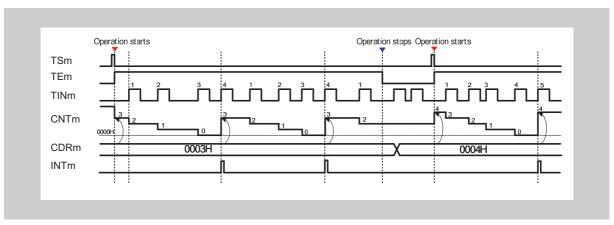
Figure 14-59 Operation stop and restart, TAUBnCMURm.TIS[1:0] = 01
