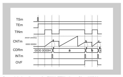
Figure 15-36 General timing diagram for TAUJnTTINm Input Signal Width Measurement Function
