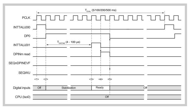
Figure 9-5 Wake-up Sequencer operation in digital input mode - no DPINm change
