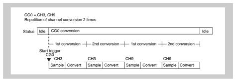
Figure 22-5 2 times repetition of channel conversion in one-shot conversion mode
