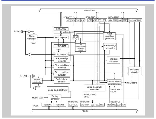
Figure 20-2 Block diagram of IICBn
