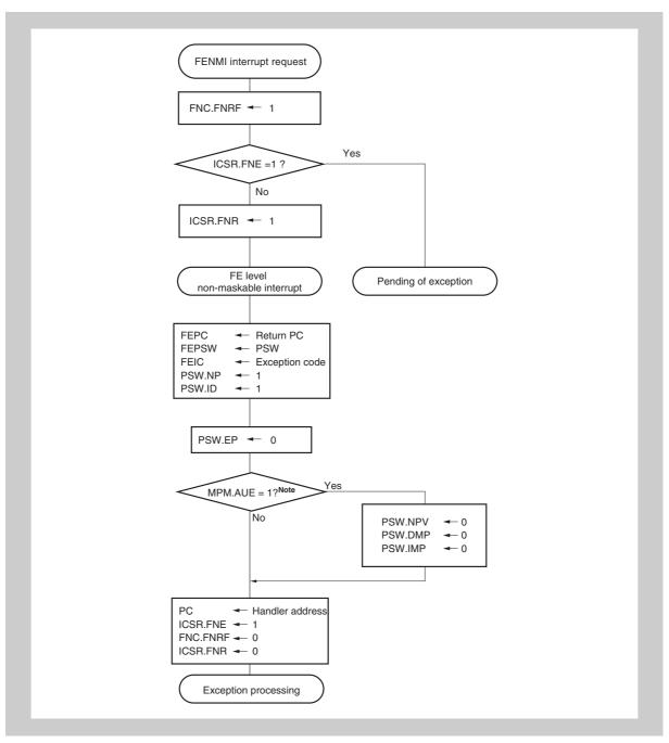
Figure 4-1 Processing upon occurrence of FENMI interrupt request
