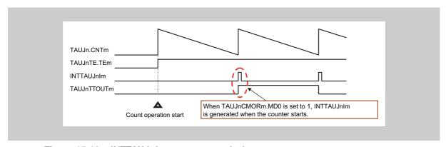
Figure 15-10 INTTAUJnIm not generated when counter starts
