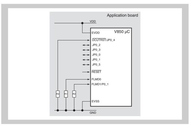
Figure 3-6 Pin connections in normal operation mode
