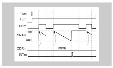
Figure 14-44 General timing diagram for Overflow Interrupt Output Function (During TAUBnTTINm Width Measurement)
