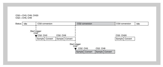
Figure 22-4 Wait until A/D conversion of current channel has been completed (ADAAnCTL1.ADAAnTRM0 = 1)
