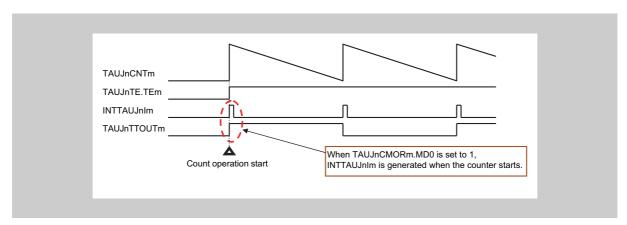
Figure 15-9 INTTAUJnIm generated when counter starts
