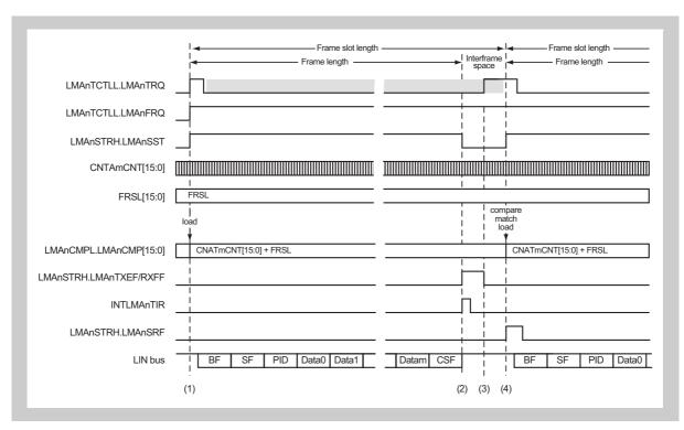
Figure 17-12 LIN frame transmission with scheduler and automatic frame start function
