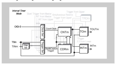
Figure 15-26 Block diagram for TAUJnTTINm Input Interval Timer Function
