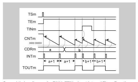
Figure 15-27 General timing diagram for TAUJnTTINm Input Interval Timer Function
