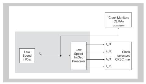
Figure 7-5 Low Speed Internal Oscillator clock generator
