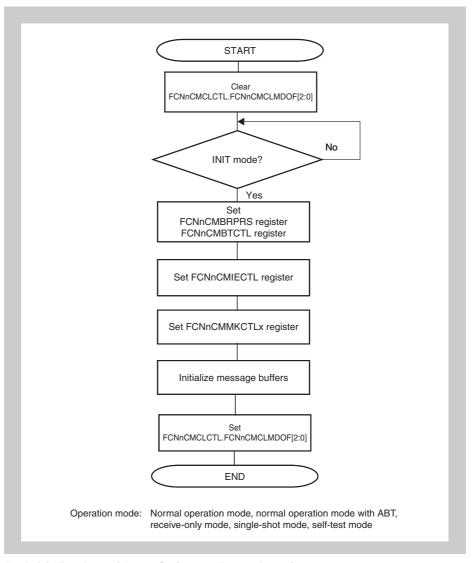
Figure 18-17 Re-initialization without Software Reset function
