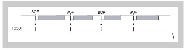
Figure 18-14 Timing diagram of capture signal TSOUT
