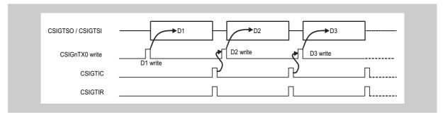
Figure 19-14 Generation of CSIGTIC after communication (CSIGnCTL1.CSIGnSLIT = 0)
