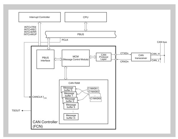
Figure 18-3 Block diagram of the CAN Controller
