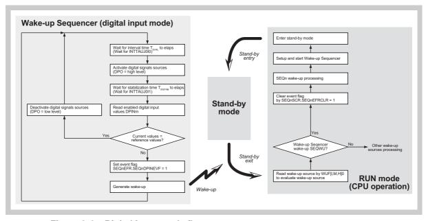
Figure 9-4 Digital input mode flow
