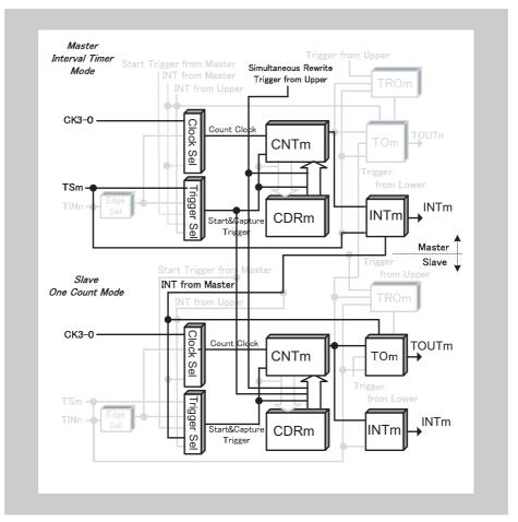
Figure 14-69 Block diagram for PWM Output Function
