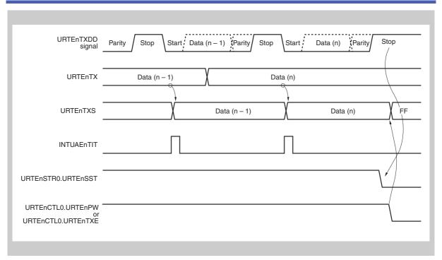
Figure 16-15 Continuous transmission operation timing - transmission end
