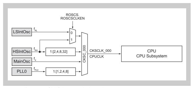
Figure 3-4 CPU Subsystem clock supply
