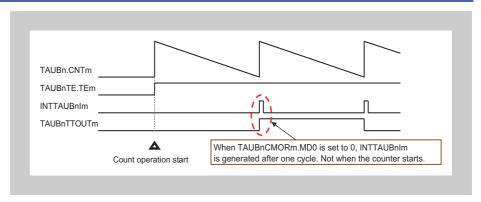
Figure 14-17 INTTAUBnlm not generated when counter starts
