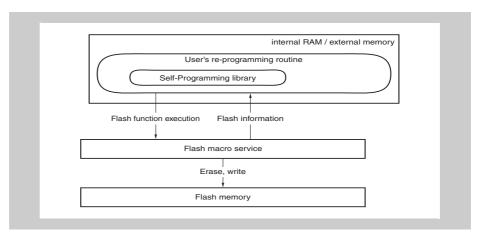
Figure 6-10 **Concept of Self-Programming**
