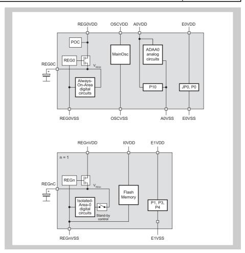
Figure 24-2 V850E2S/FF4-L power supply scheme
