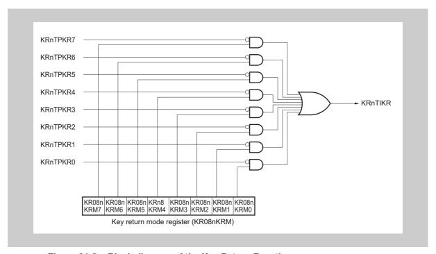
Figure 21-2 Block diagram of the Key Return Function
