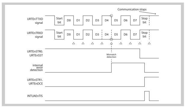
Timing example of data consistency error (no BF reception active, i.e. **Figure 16-11** URTEnSTR0.URTEnSSBR = 0)
