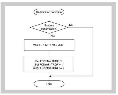
Figure 18-6 Setting transmission request (FCNnMmCTL.FCNnMmTRQF) to transmit message buffer after redefinition
