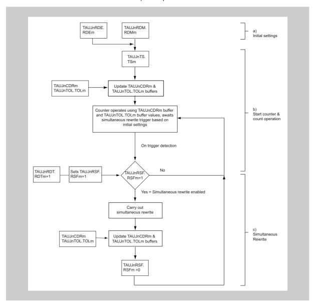
Figure 15-4 General procedure for simultaneous rewrite
