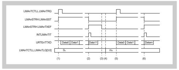
Figure 17-4 Data transmission in UART buffer mode
