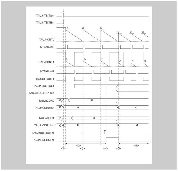
Figure 15-5 Simultaneous rewrite when the master channel (re)starts counting
