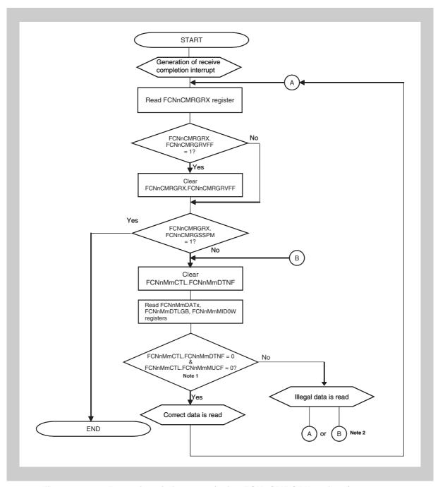
Figure 18-35 Reception via interrupt (using FCNnCMRGRX register)
