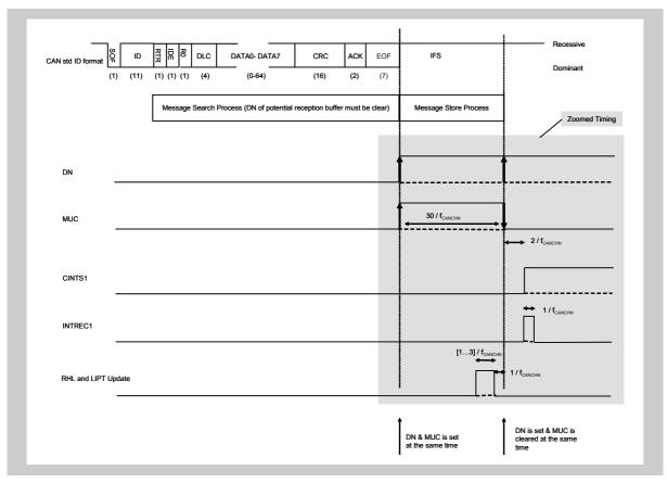
Figure 18-8 FCNnMmCTL.FCNnMmDTNF and FCNnMmCTL.FCNnMmMUCF bit setting period (for standard ID format)
