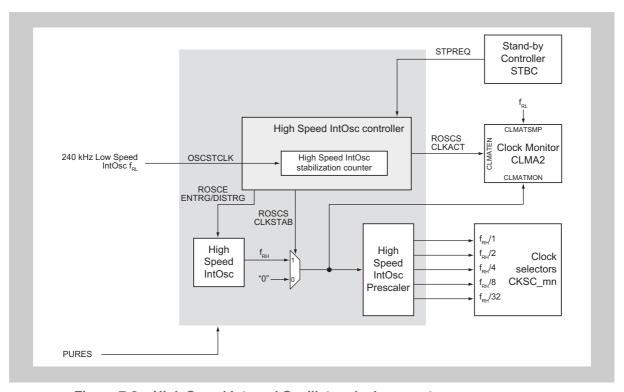
Figure 7-6 High Speed Internal Oscillator clock generator
