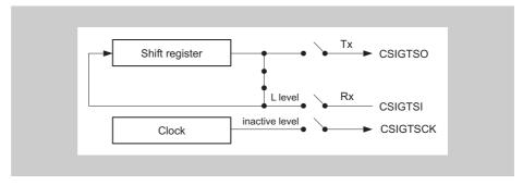
Figure 19-22 Operation in loop-back mode
