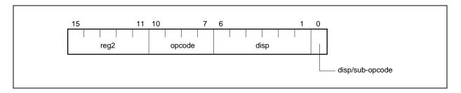
A 16-bit instruction format having a 7-bit opcode field, a general-purpose register specification field, and a 4-bit displacement field.
