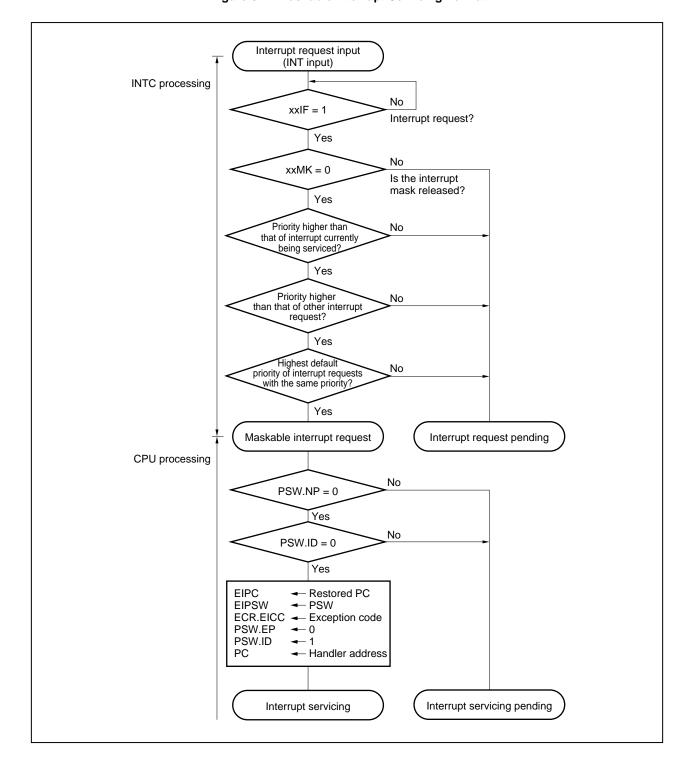
Figure 6-1. Maskable Interrupt Servicing Format
