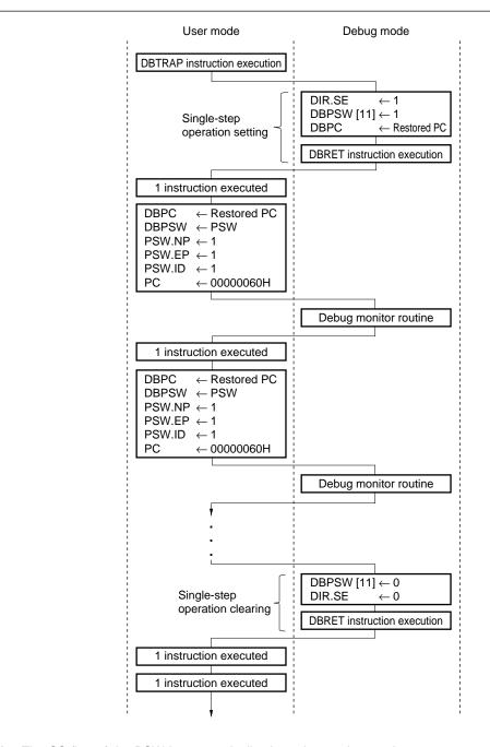
Figure 9-1. Single-Step Operation Execution Flow
