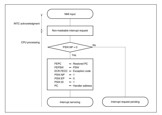
Figure 6-2. Non-Maskable Interrupt Servicing Format
