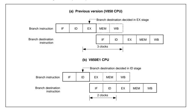
Figure 8-4. Pipeline Operations with Branch Instructions
