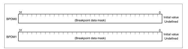
Figure 2-16. Breakpoint Data Mask Registers 0 and 1 (BPDM0, BPDM1)
