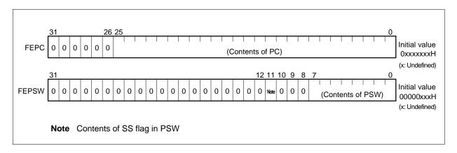
Figure 2-4. NMI Status Saving Registers (FEPC, FEPSW)
