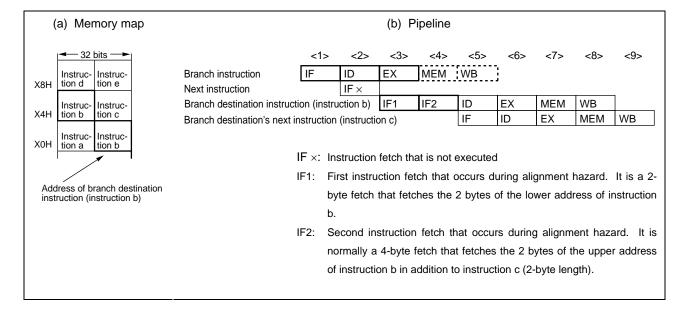
Figure 8-6. Alignment Hazard Example
