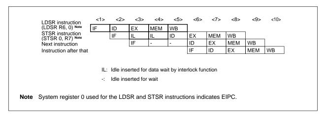
As shown in Figure 8-9, when an STSR instruction is placed immediately after an LDSR instruction that uses the operand EIPC or FEPC, and that STSR instruction uses the LDSR instruction execution result, the interlock function causes a data wait time to occur, and the execution speed is lowered. This drop in execution speed can be avoided by placing STSR instructions that reference the execution result of the preceding LDSR instruction at least 3 instructions after the LDSR instruction.
