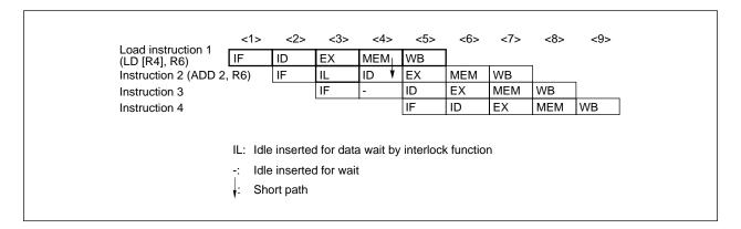
Figure 8-7. Example of Execution Result of Load Instruction
