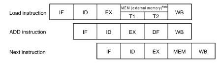
**Note** The basic bus cycle for the external memory of MEMC is 2 clocks.
