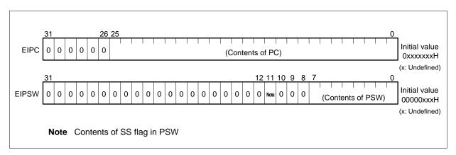
Figure 2-3. Interrupt Status Saving Registers (EIPC, EIPSW)
