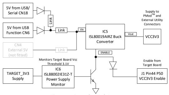
Figure 4-1: Power Supply Scheme
