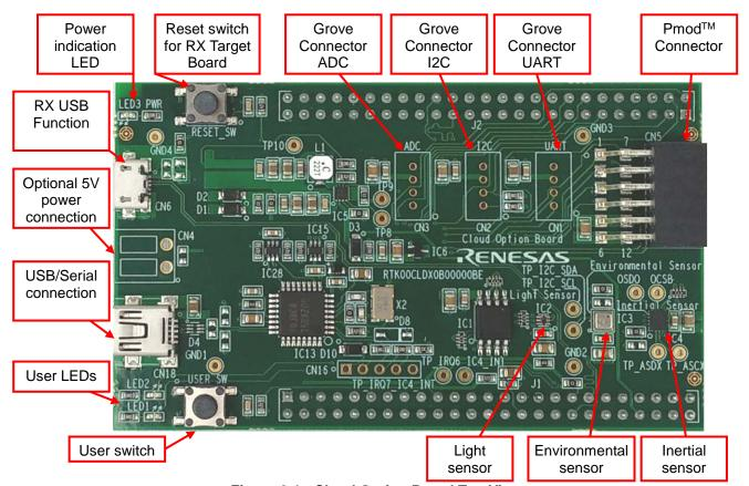
Figure 2-1: Cloud Option Board Top View
