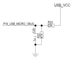
Figure 4-3: USB\_VBUS signal to Target Board MCU
