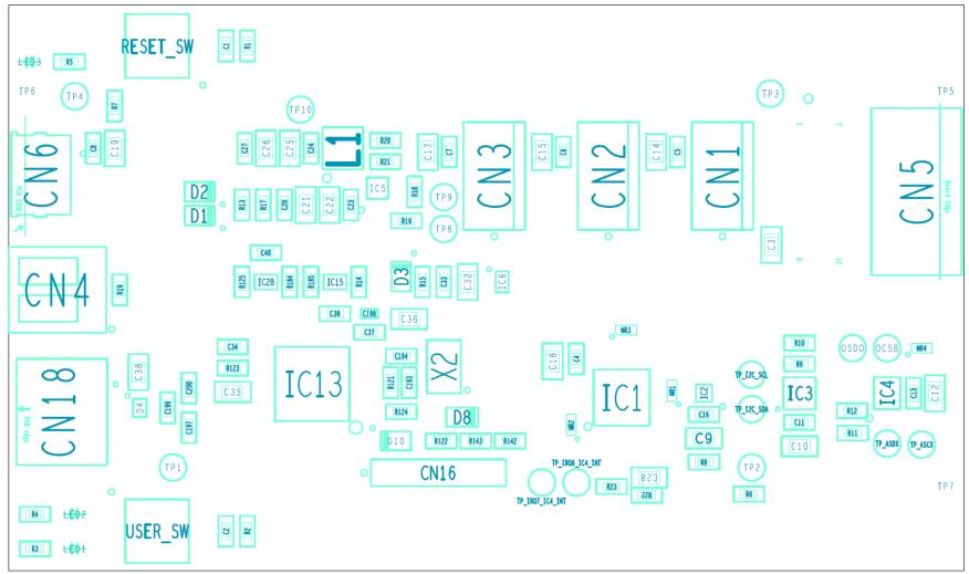
Figure 3-1 : Component Positions on Top Side of Board
