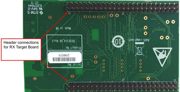
Figure 2-2: Cloud Option Board Bottom View
