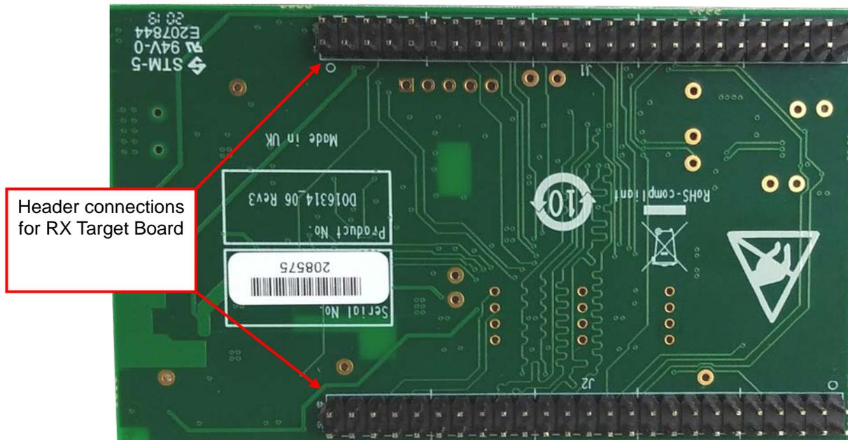
Figure 2-2 : Cloud Option Board Bottom View
