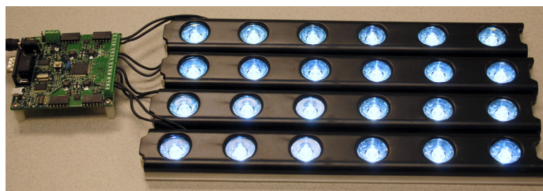
Figure 5: Driving the Dialight Light Engines
