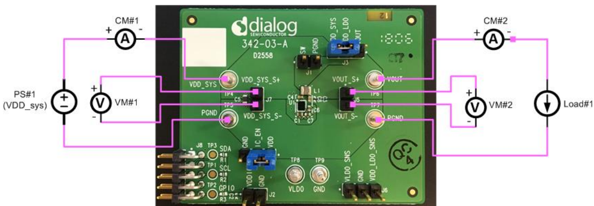
Figure 4: Recommended Setup for Buck Efficiency Measurement
