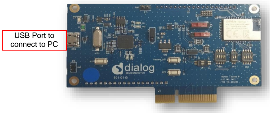
Figure 1: UART Connection with PC via USB Port at DA16200 EVB
