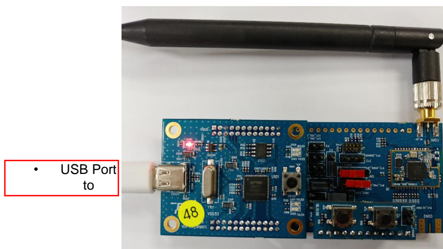
Figure 1: UART Connection with PC via USB Port
