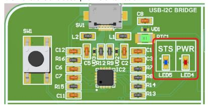
Figure 3: Connection Status and Power LEDs
