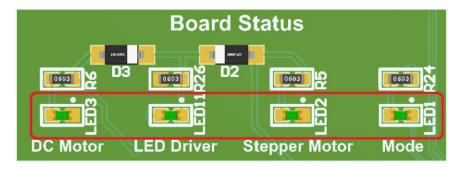
Figure 4: Board Status LEDs
