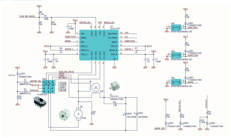
Figure 18: HV PAK Main Circuit
