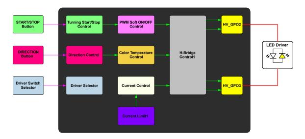
Figure 12: LED Driver Functional Block Diagram
