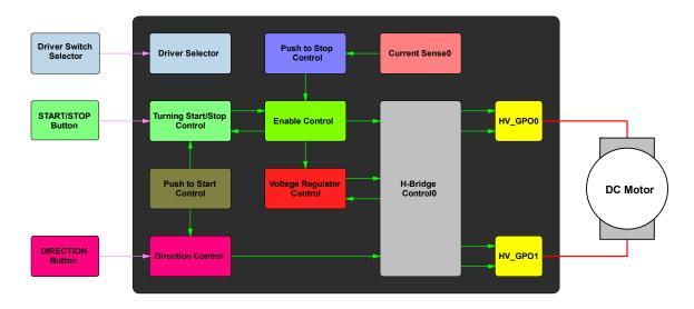
Figure 10: DC Motor Driver Functional Block Diagram
