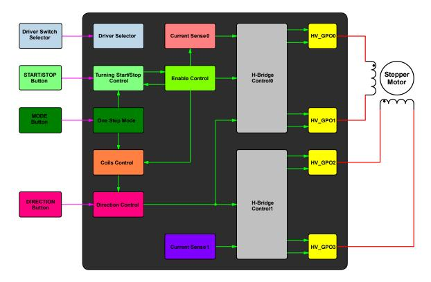
Figure 11: Stepper Motor Driver Functional Block Diagram
