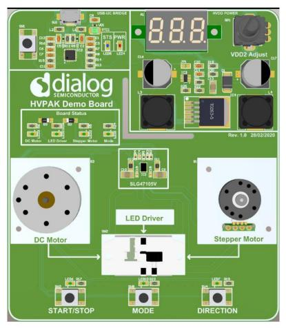
Figure 1: SLG47105 Demo Board General View
