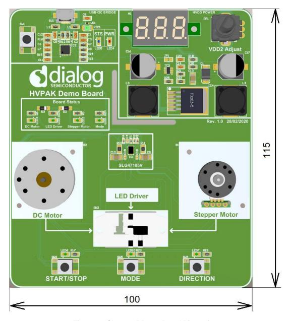
Figure 13: SLG47105 Demo Board Dimensions
