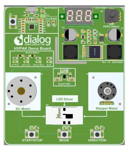
Figure 14: SLG47105 Demo Board, Top View
