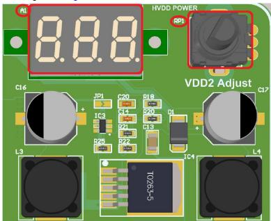
Figure 2: HV<sub>DD</sub> Voltage Indicator and Regulator
