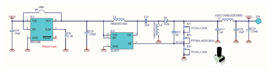
Figure 17: HV<sub>DD</sub> Power Supply
