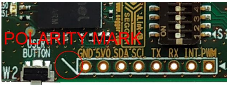
Figure 18. Guides for proper MikroBUS™ click board insertion
