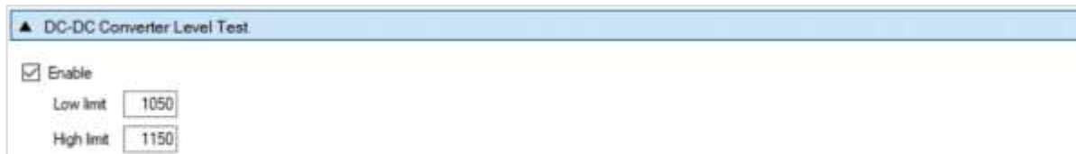
Figure 53: DC-DC Converter Level Test - DA1453x
