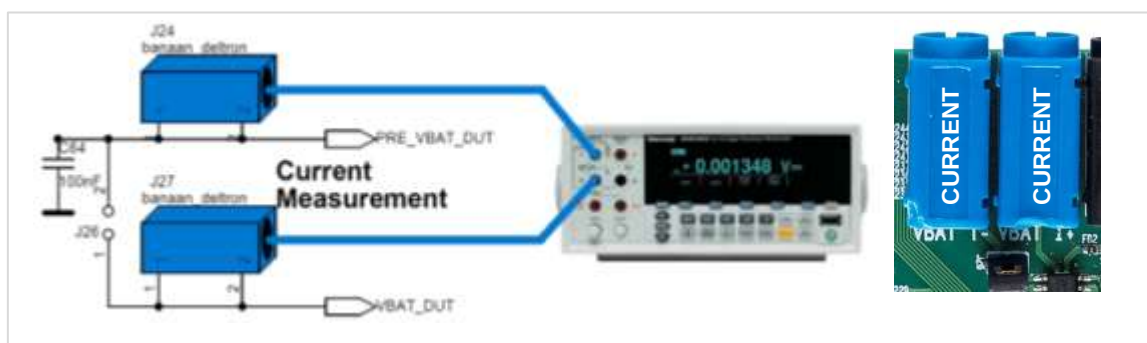
Figure 12: VBAT DUT current measurement setup
