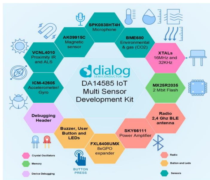
Figure 2: DA14585 IoT MSK Block Diagram
