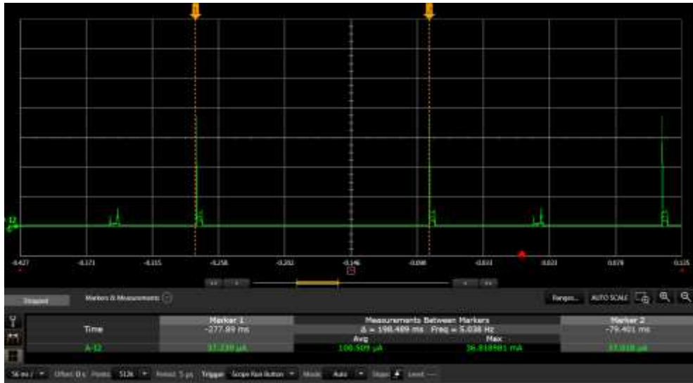
Figure 29: DA14585 Voice RCU Reference Design – Average Touch Pad Scanning Current
