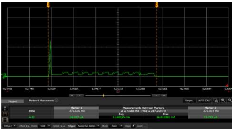
Figure 30: DA14585 Voice RCU Reference Design – Current during Touch Pad Scan Pulse
