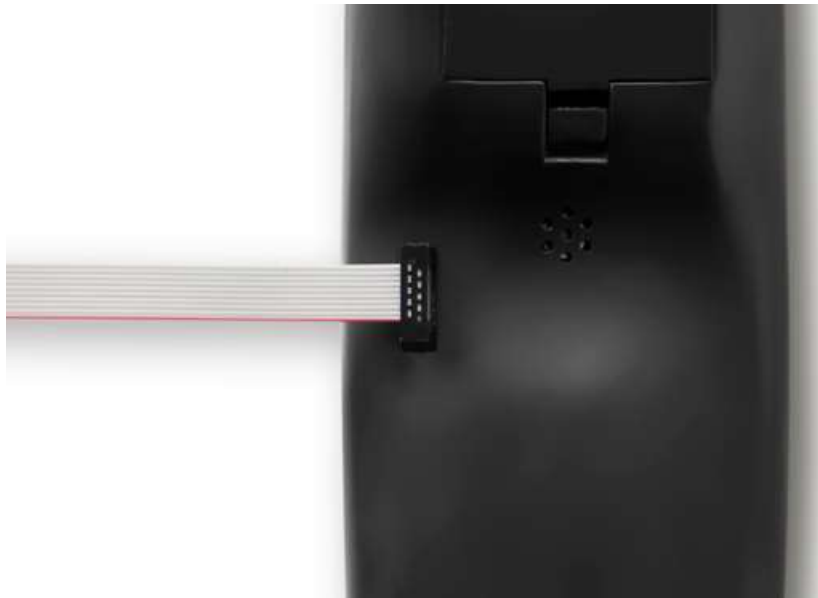
Figure 33: Connection of JTAG Cable with DA14585 Voice RCU PCB Inside Enclosure
