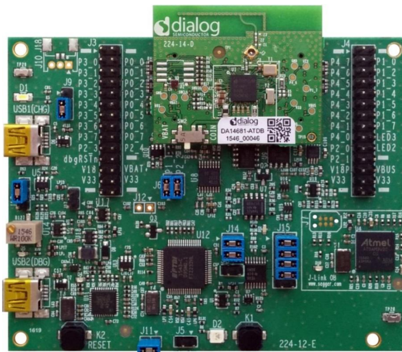
Figure 11 Pro DK Jumper Placement for Full UART Functionality
