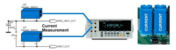
Figure 11: VBAT DUT Current Measurement Setup
