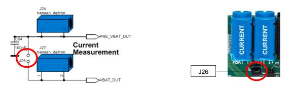
Figure 12: Connections for 'Floating Current' Measurements
