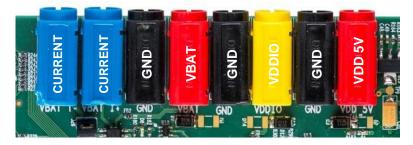
Figure 4: PLT Hardware Power Connections
