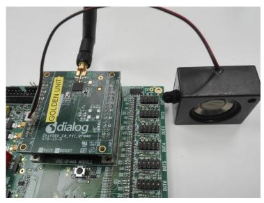
Figure 144: Speaker Connection for Audio Test.
