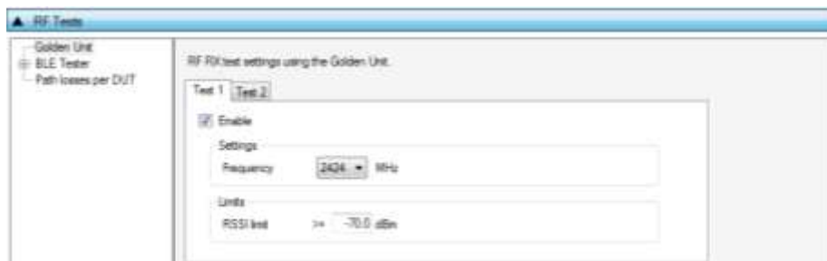
Figure 12: DA1458x_DA1468x_CFG_PLT.exe with Two GU RF Tests
