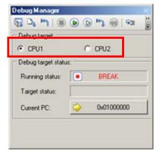
Here, the state of CPU1 being selected should not be changed.
