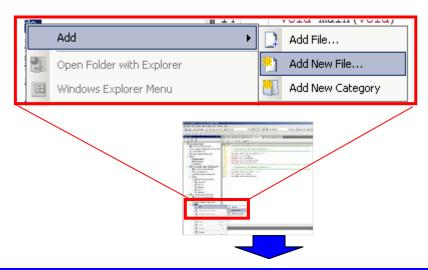
Add the following two files. Set the C1H\_sample\u22a4C1H\_sample\_App1 folder as the place where the files are to be created.
