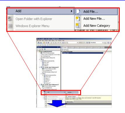
Select the assembly source file, open C1H\_sample\_App1 and DefaultBuild, and then select "C1H\_sample\_App1.fsy" to add the file.
