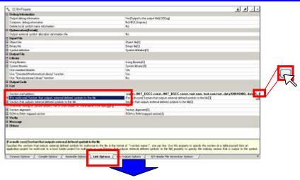
This opens the [Section Settings] dialog box. Click the [Add] button to add three sections "com.text", "com.bss", and "com.data". Then make and edit settings as shown below.
