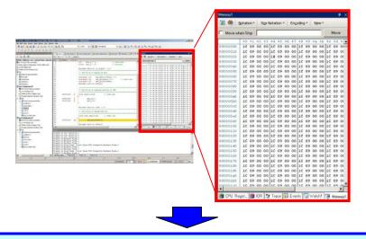
Make the Memory 2 panel enter the floating state and dock it to the Output panel.
