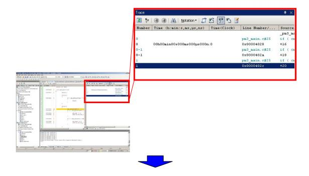
Settings for tracing can be made in the [Trace] category on the [Debug Tool Settings] tab of the Property panel. Select the [Debug Tool Settings] tab and make the settings as shown below.
