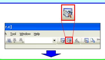
Check to see if the rebuild process has been completed correctly. If the build process has been completed correctly, a load module file is created.
