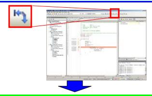
The program breaks at the line where the break has been set and the breakpoint line is highlighted in yellow.
