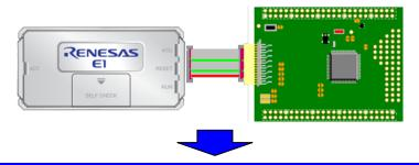
Connect E1 to the PC. ("Found New Hardware Wizard" appears when E1 is connected for the first time. Select "Install software automatically" and install the USB driver following the instructions.)
