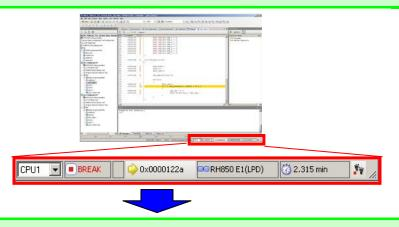
The source code line where the program stopped (current position of the program counter (PC)) is highlighted in yellow.
