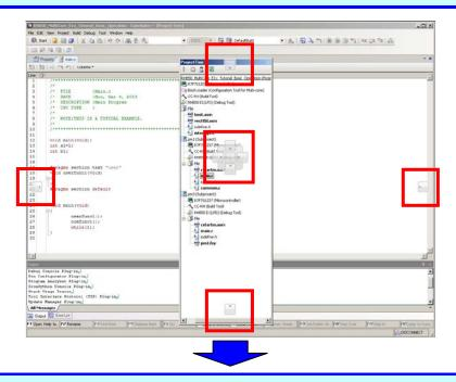
Place the pointer on the navigation icon located in the desired destination location and the destination area is highlighted in blue.
