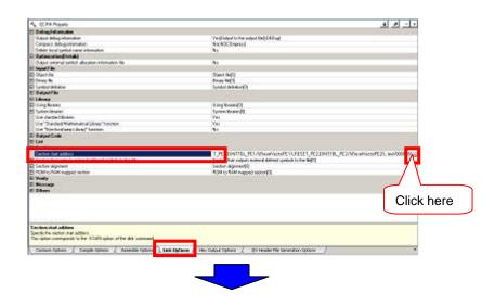
This opens the [Section Settings] dialog box. Select "%ResetVectorPE2%" and click the [Remove] button.
