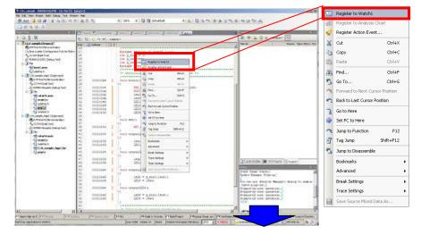
This opens the Watch panel where you can confirm that the variable is now registered. The current value of "g\_counter" is ?.
