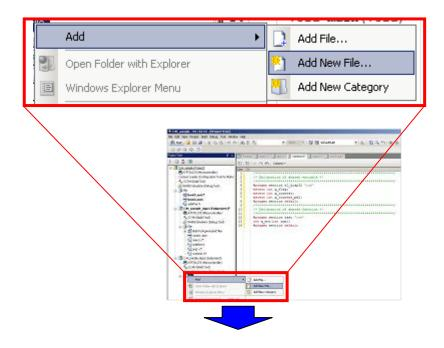
Add the following two files. Set the C1H\_sample\(\text{YC1H\_sample\_App2}\) folder as the place where the files are to be created.
