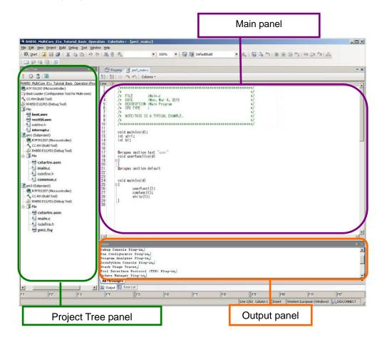
Project Tree panel: Displays the functions of CS+ corresponding to the flow of system development.
