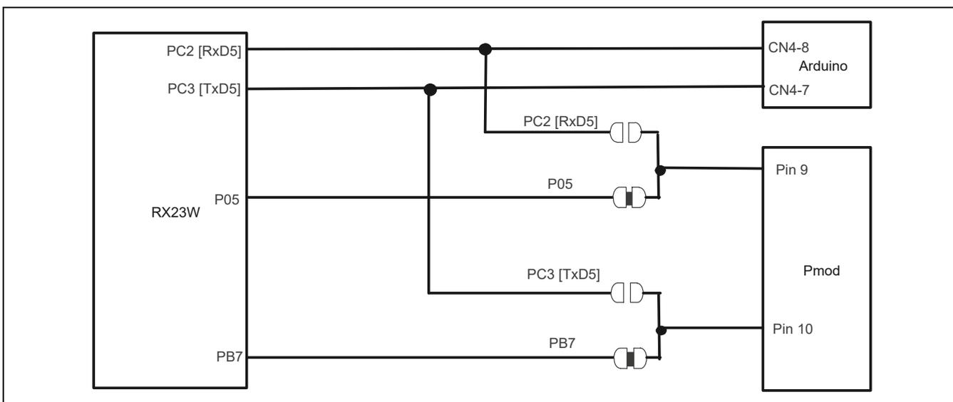
Figure 5-7 Pmod™ Multi-Function Pins
