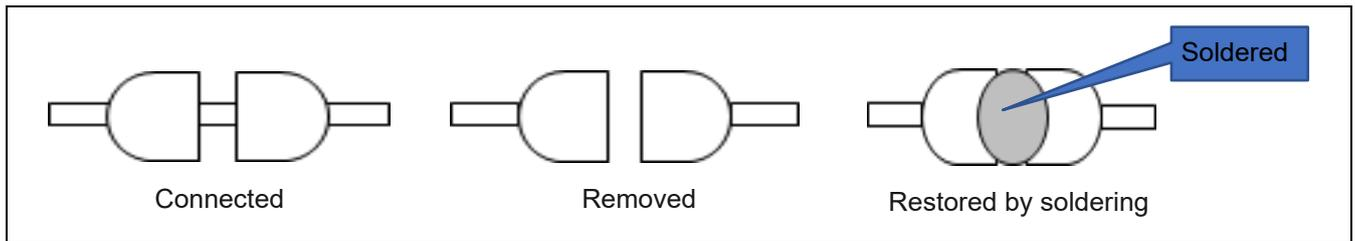
Figure 5-9 Examples of States of Patterns for Cutting
