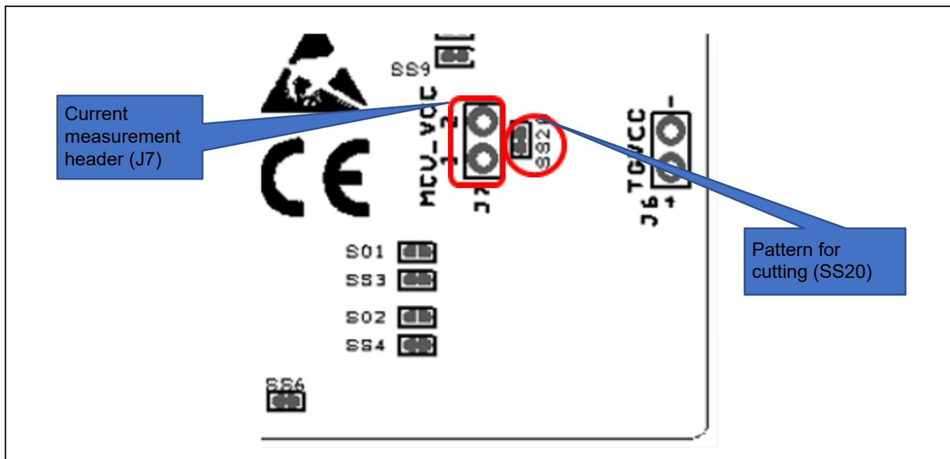
Figure 5-8 Positions of the Current Measurement Header (J7) and Pattern for Cutting (SS20) (Soldered Side)
