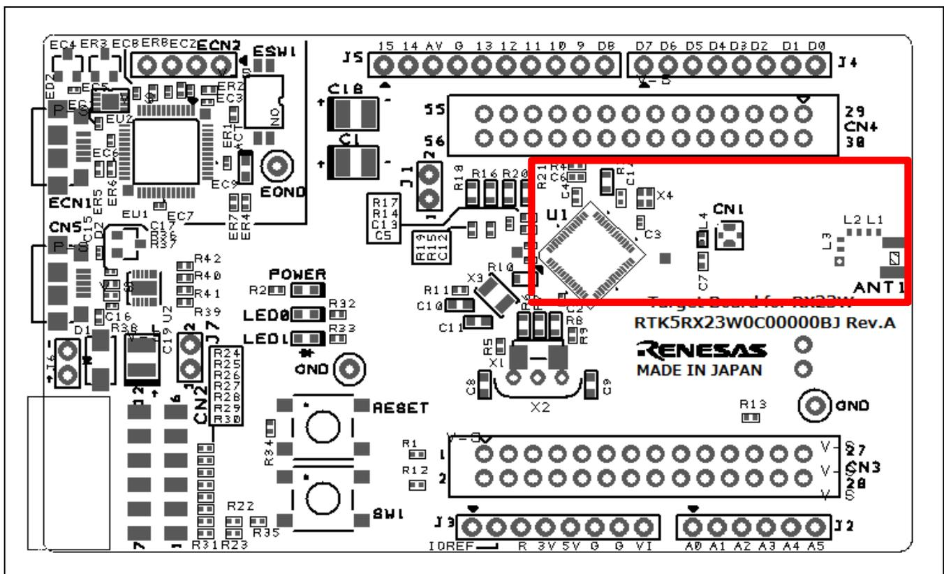
Figure 5-1 BLE Circuit
