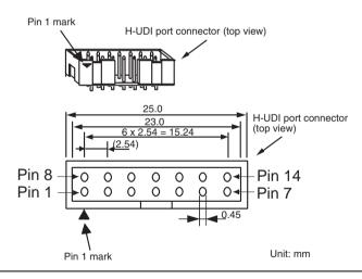
Figure 1.1 Pin Assignments of the H-UDI Port Connector
