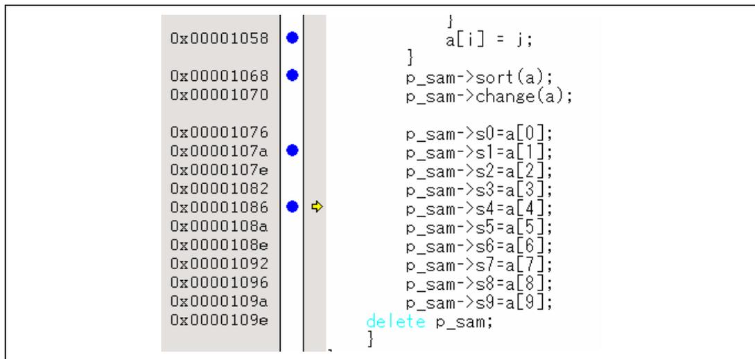
The image shows a source code window with a list of memory addresses on the left and corresponding C code on the right. A yellow arrow points to the line `p_sam->s4=a[4];` at address `0x00001086`, indicating a sequential break. The code is as follows:
