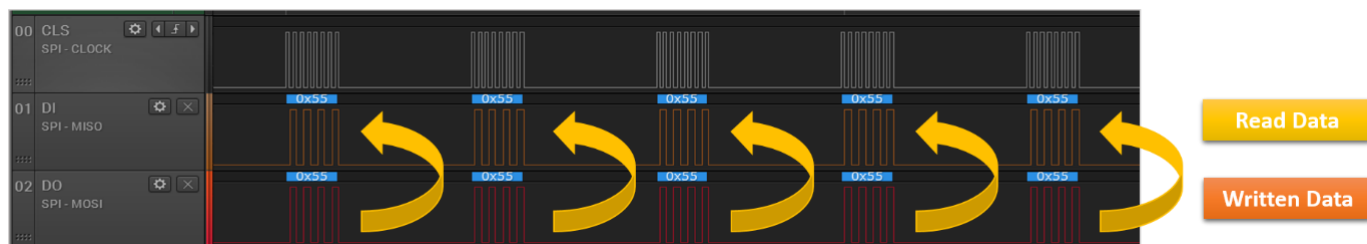
Figure 18: SPI Duplex Transaction Captured using a Logic Analyzer.
