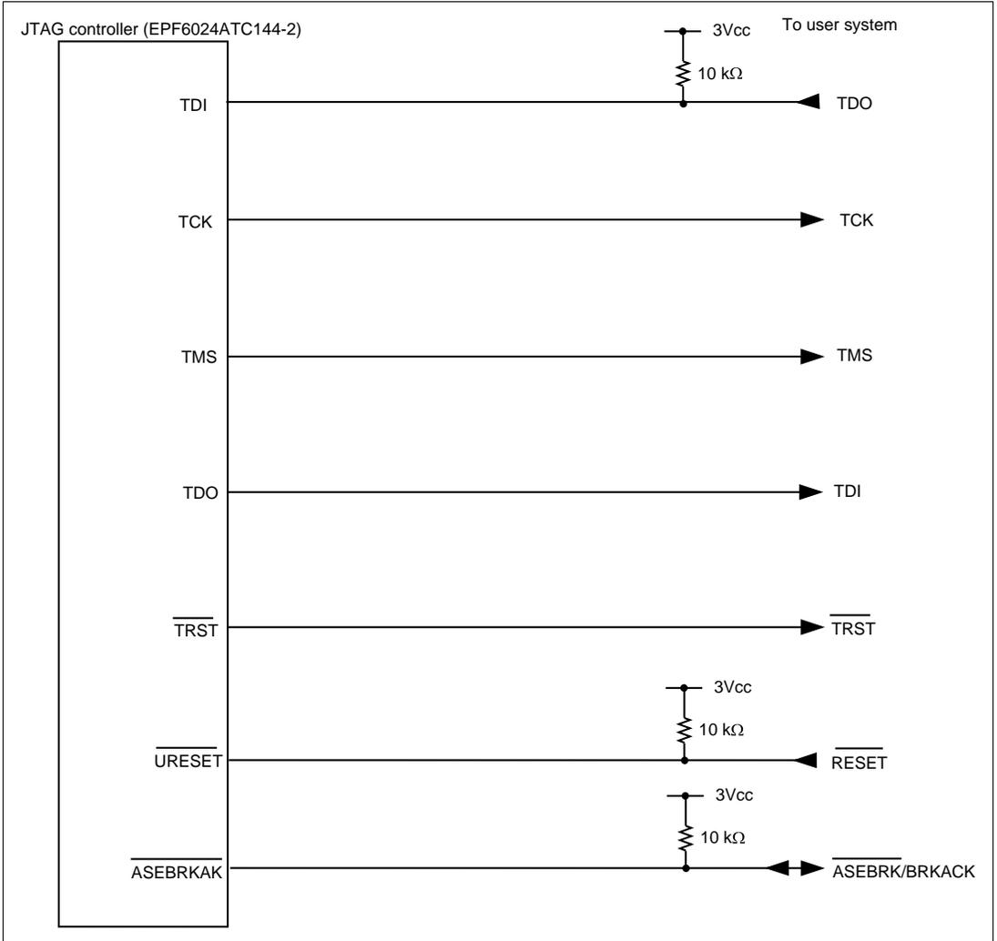
**Figure 6.5 User System Interface Circuit of the Hitachi-UDI Pin (HS7760KCM02H)
