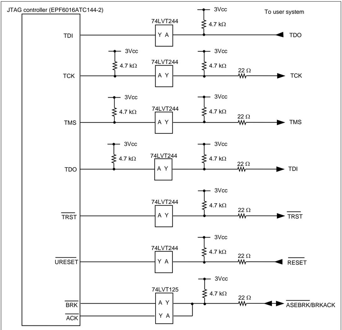
**Figure 6.4 User System Interface Circuit (HS7760KCM01H)**
