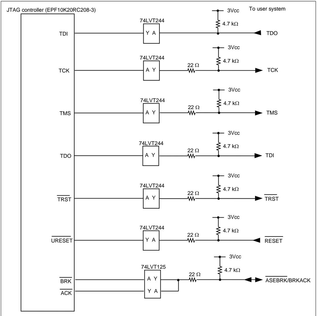
**Figure 6.7 User System Interface Circuit (HS7760KCI01H)**
