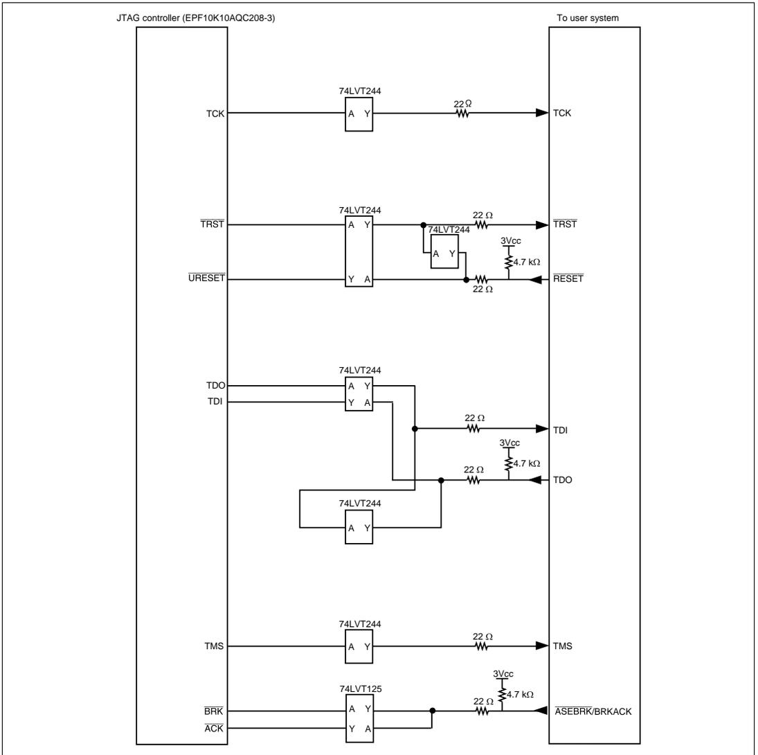
**Figure 6.8 User System Interface Circuit of the Hitachi-UDI Pin (HS7760KCI02H)
