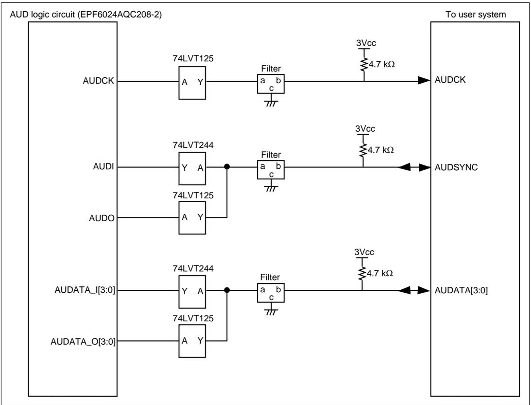
**Figure 6.9 User System Interface Circuit of the AUD Pin (HS7760KCI02H)
