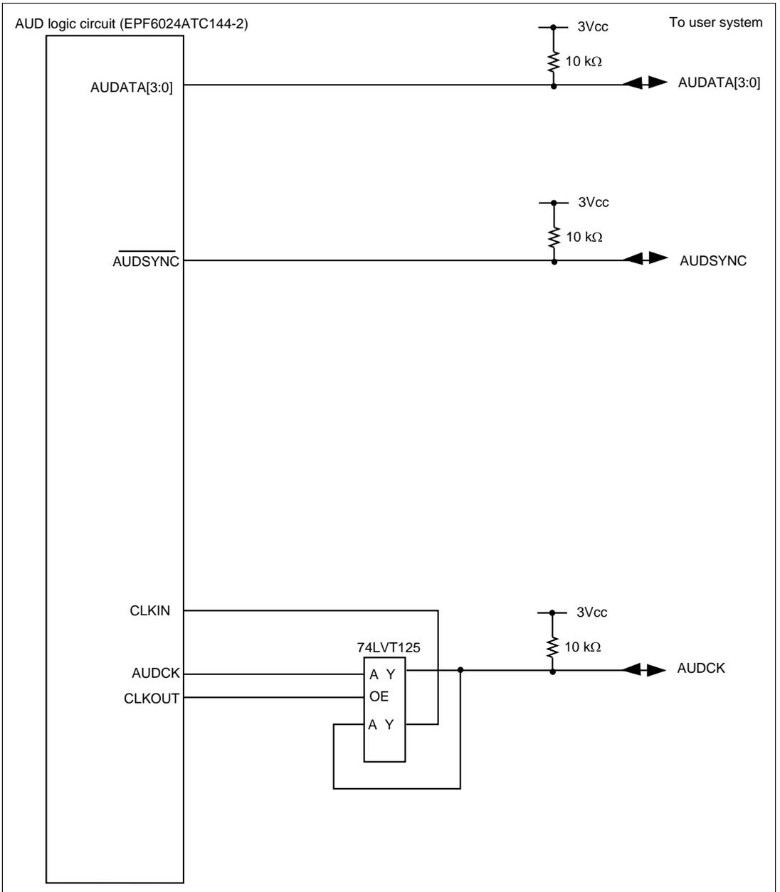
**Figure 6.6 User System Interface Circuit of the AUD Pin (HS7760KCM02H)
