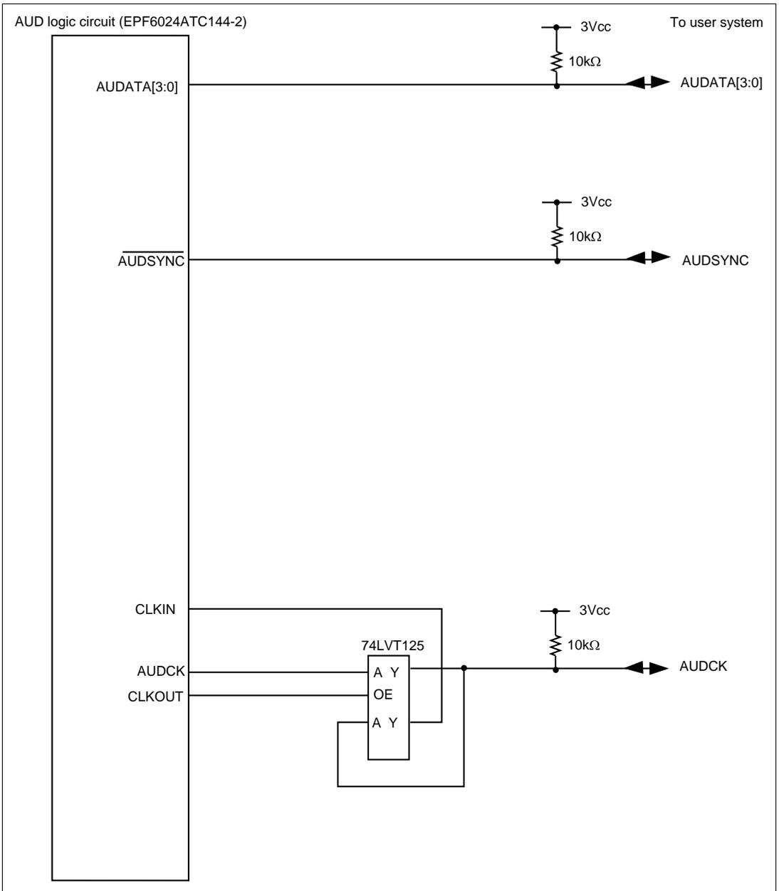
**Figure 6.6 User System Interface Circuit of the AUD Pin (HS7705KCM02H)
