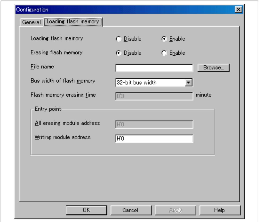
Figure 4.5 [Loading flash memory] Page ([Configuration] Dialog Box)
