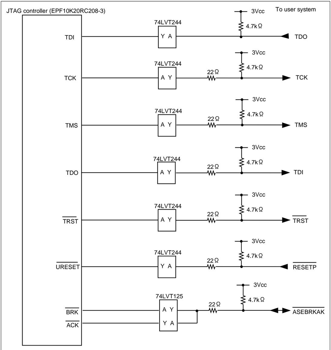
**Figure 6.7 User System Interface Circuit (HS7705KCI01H)**
