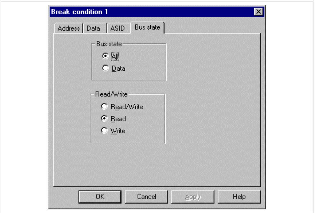
**Figure 3.45 [Bus State] Page ([Break Condition 1] Dialog Box)**
