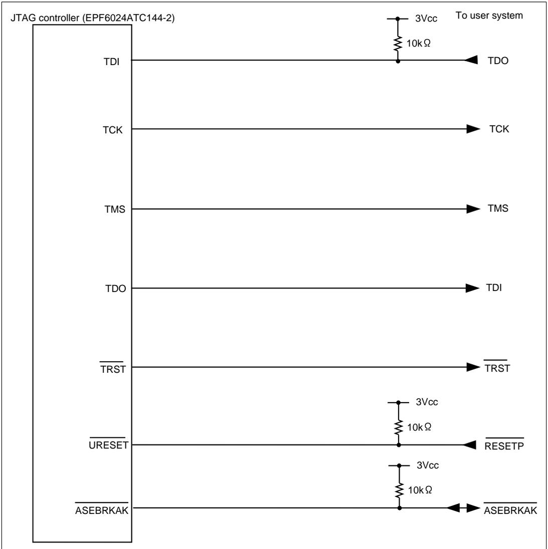
**Figure 6.5 User System Interface Circuit of the Hitachi-UDI Pin (HS7705KCM02H)
