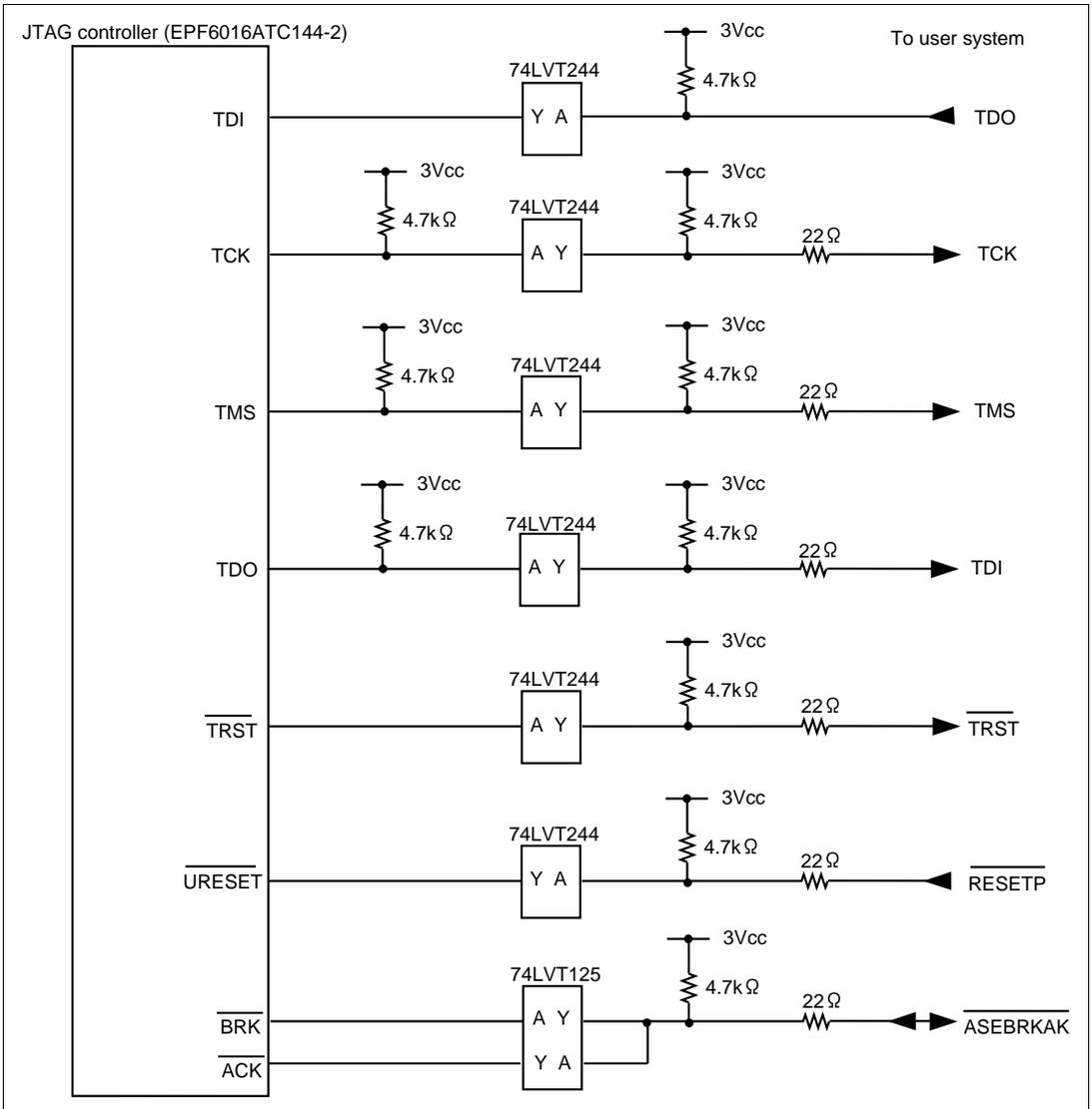
**Figure 6.4 User System Interface Circuit (HS7705KCM01H)
