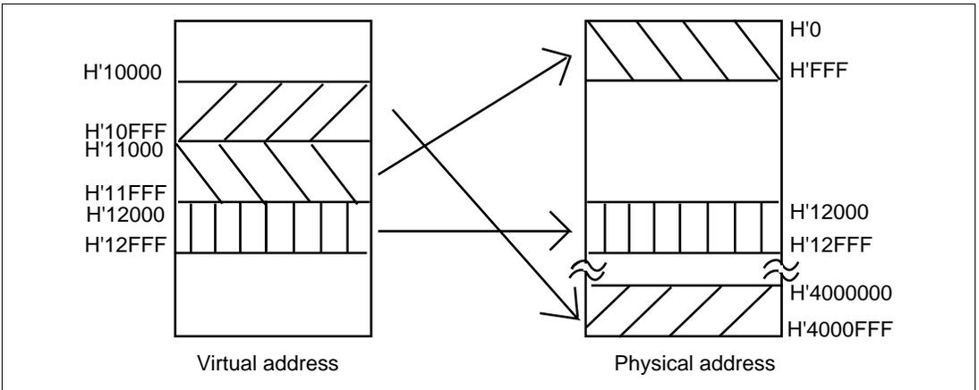
**Figure 3.58 Address Translation according to VP\_MAP Tables**
