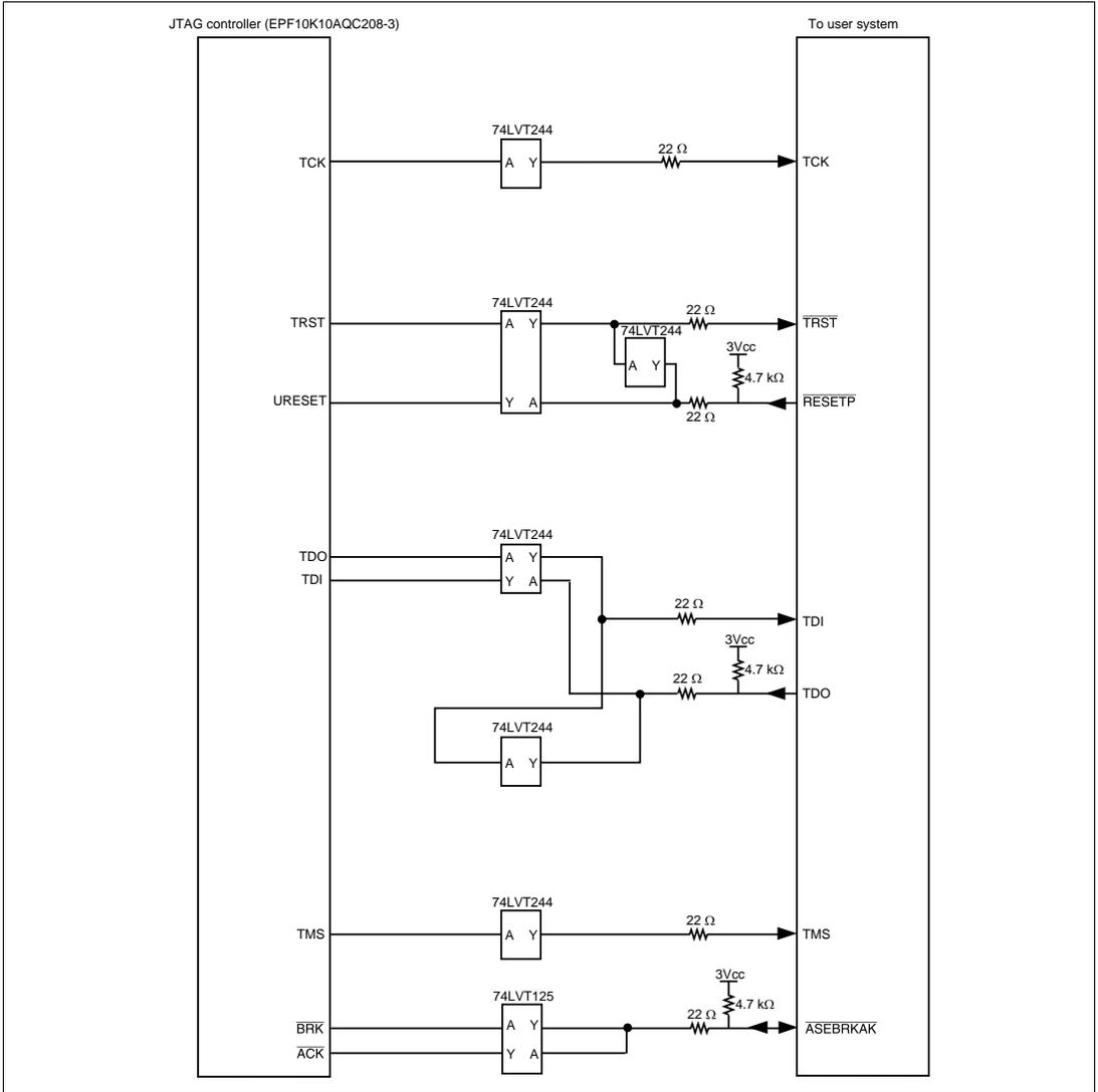
**Figure 6.8 User System Interface Circuit of the Hitachi-UDI Pin (HS7705KCI02H)
