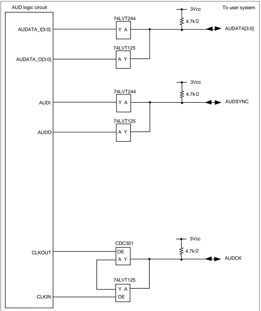
**Figure 6.9 User System Interface Circuit of the AUD Pin (HS7705KCI02H)
