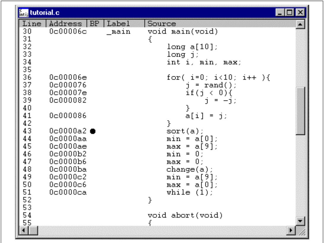
Figure 3.10 [Source] Window (Setting a Software Breakpoint)
