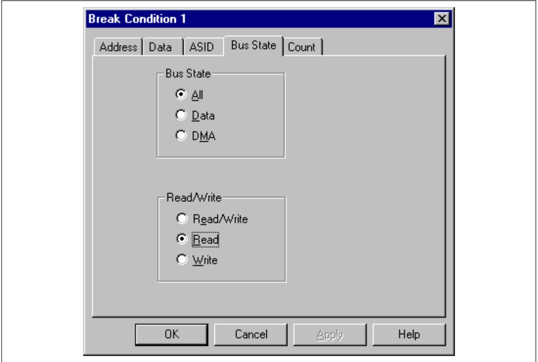
Figure 4.15 [Bus State] Page ([Break Condition] Dialog Box)
