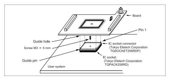
Figure 3 Connecting User System Interface Board to User System
