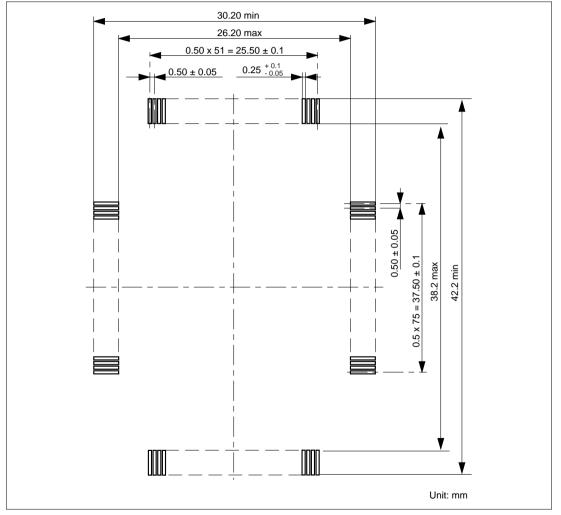
Figure 6 Recommended Dimensions for Mount Pad
