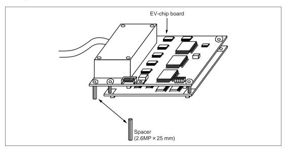
Figure 4 Exchanging the Spacer
