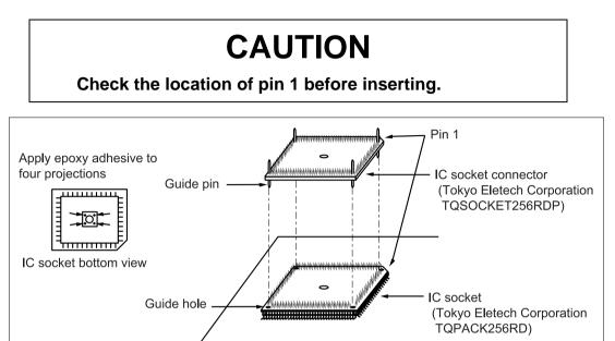
Figure 2 Installing IC Socket to User System
