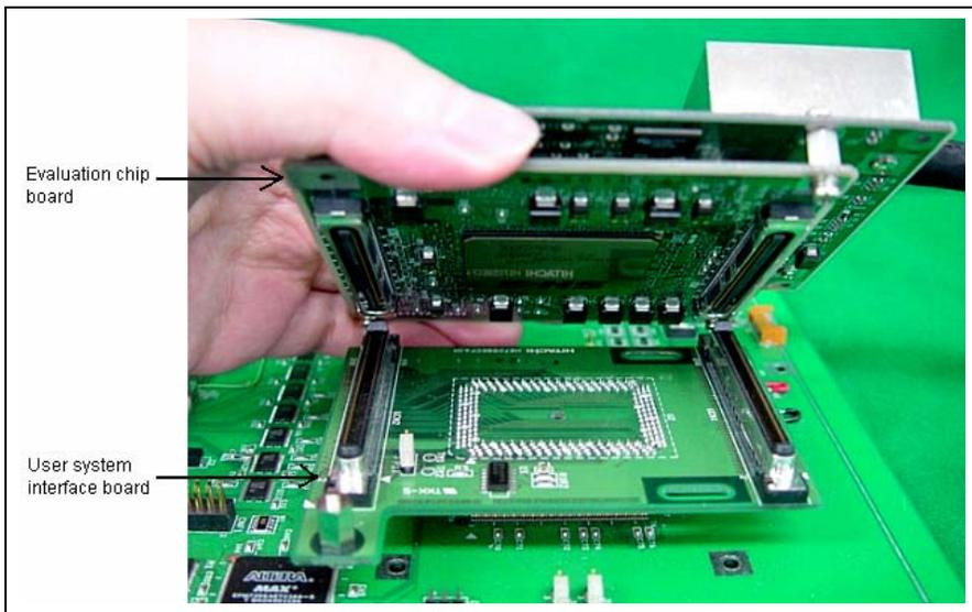
Figure 2.2 Connecting the User System Interface Board
