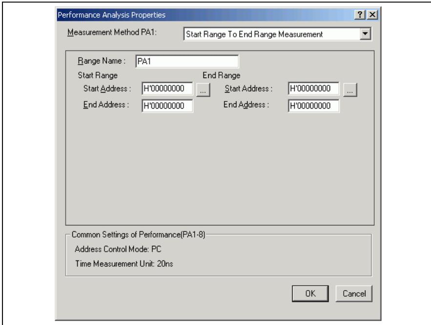
**Figure 3.38 Start Range To End Range Measurement Settings**
