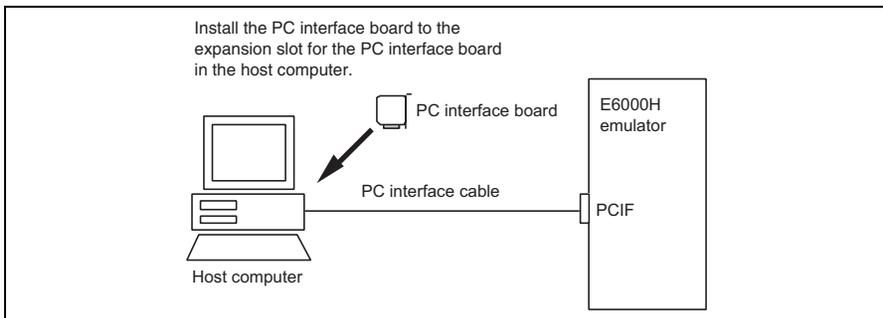
Figure 1.6 System Configuration Using a PC Interface Board
