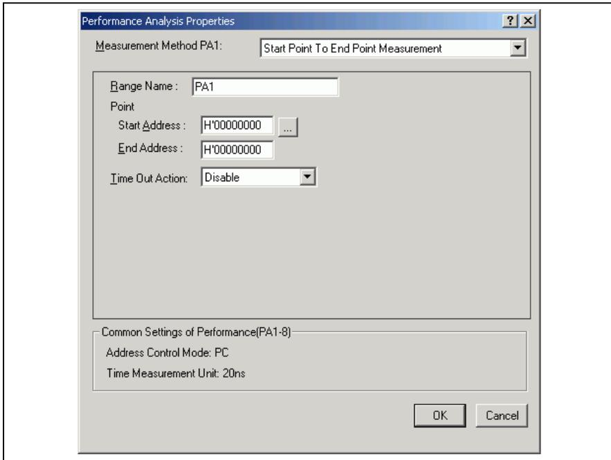
**Figure 3.37 Start Point To End Point Measurement Settings**
