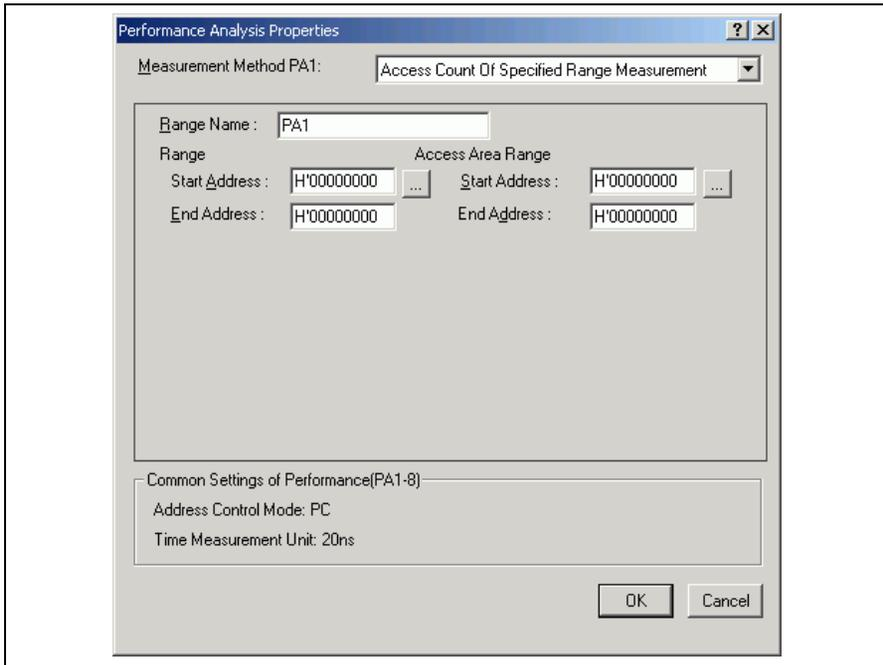
**Figure 3.39 Access Count Of Specified Range Measurement Settings**
