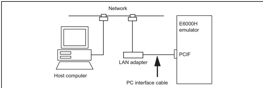
Figure 1.7 System Configuration Using a LAN Adapter
