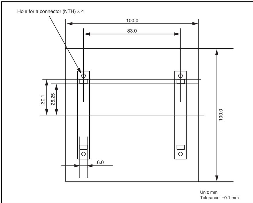
**Figure 3.17 Location for Mounting the Connector in the User System**
