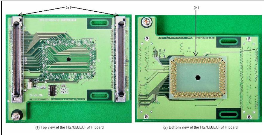
**Figure 1.5 Configuration of User System Interface Board**
