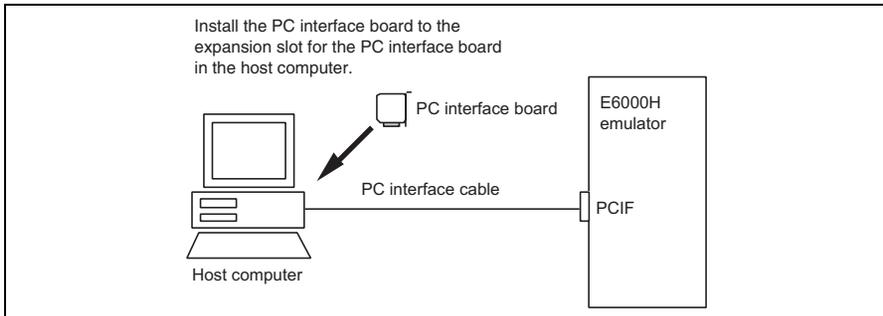
Figure 1.6 System Configuration Using a PC Interface Board
