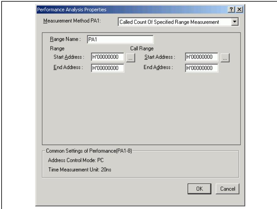
**Figure 3.40 Called Count Of Specified Range Measurement Settings**
