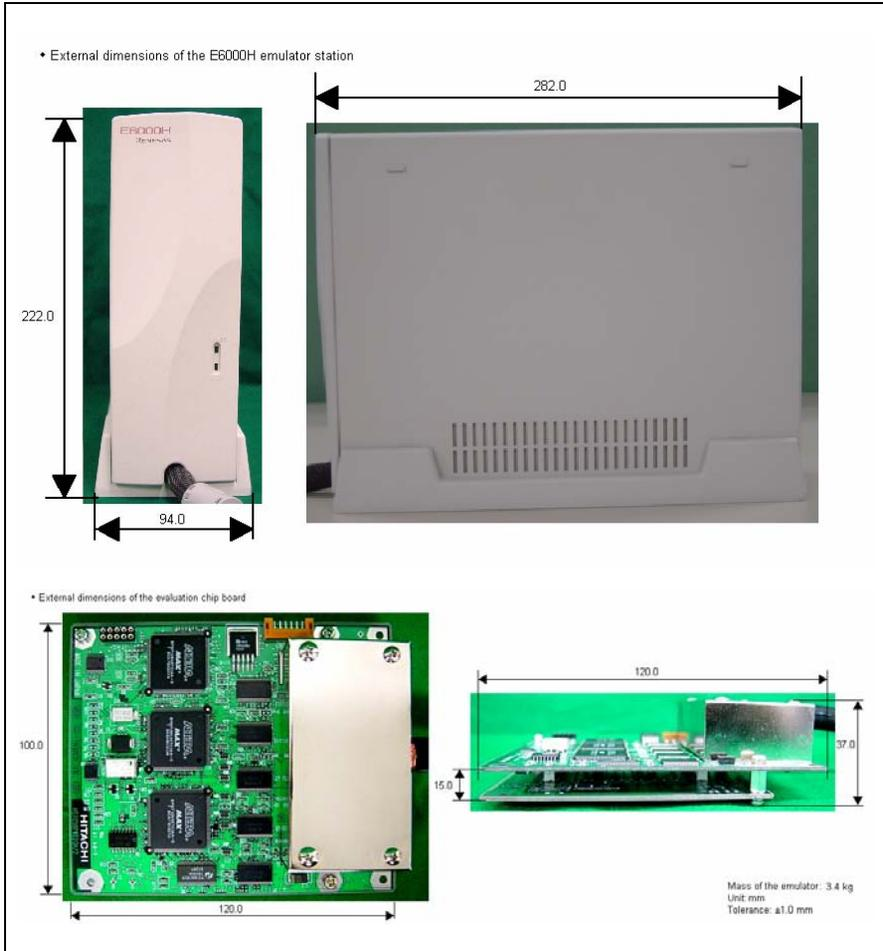
Figure 3.1 External Dimensions and Mass of the Emulator
