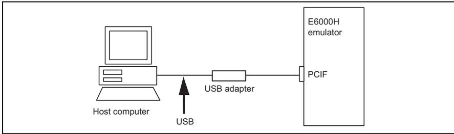
**Figure 1.8 System Configuration Using a USB Adapter**
