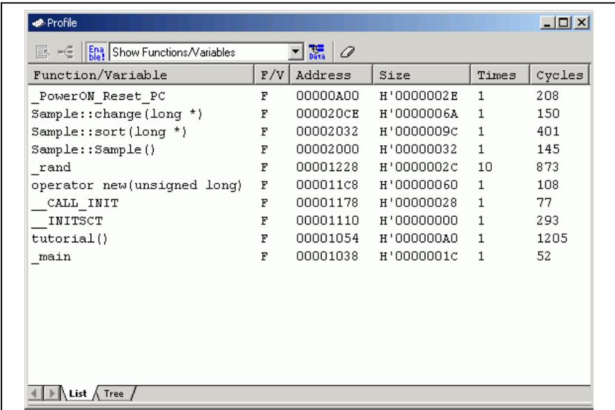
The screenshot shows a window titled "Profile" with a menu bar containing "Show Functions/Variables" and a toolbar with "Data" and "Edit" icons. Below the toolbar is a table with the following columns: "Function/Variable", "F/V", "Address", "Size", "Times", and "Cycles". The table contains the following data:
