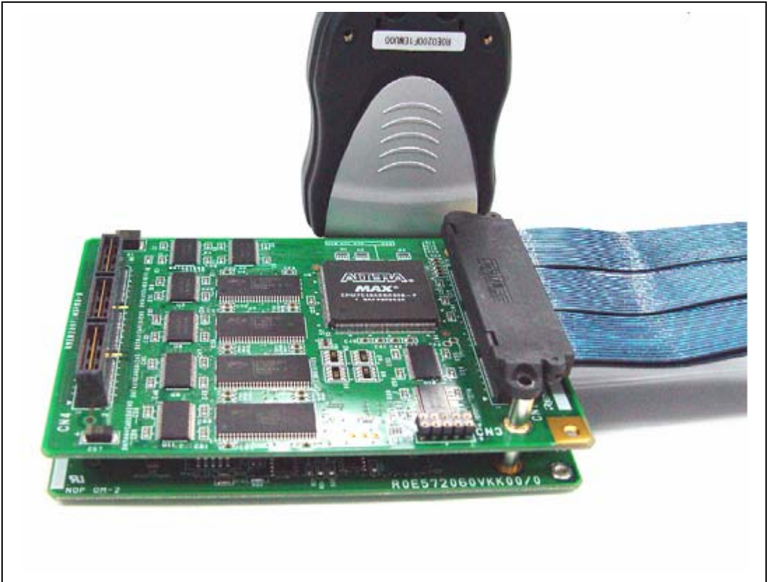
Figure 2.7 Connecting the Emulation Memory Unit, EV-chip Unit, and Trace Cable
