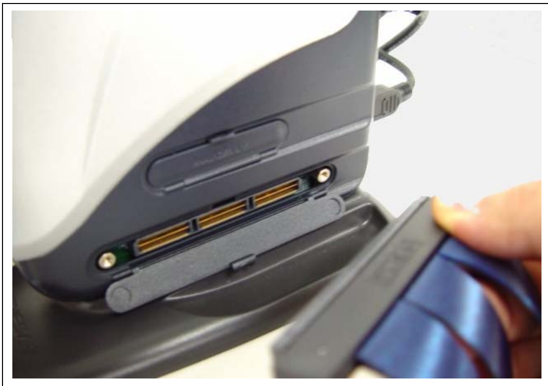
Figure 2.1 Connecting the Trace Cable to E200F when Using the EV-chip Unit
