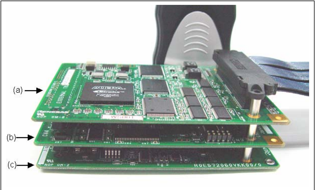
Figure 2.8 Connecting the External Bus Trace Unit, Emulation Memory Unit, and EV-chip Unit
