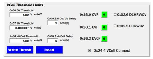
Figure 28. VCell Thresholds
