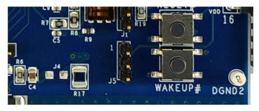
Figure 6. Communication Select Jumper
