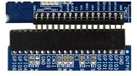
Figure 11. Dongle Connection
