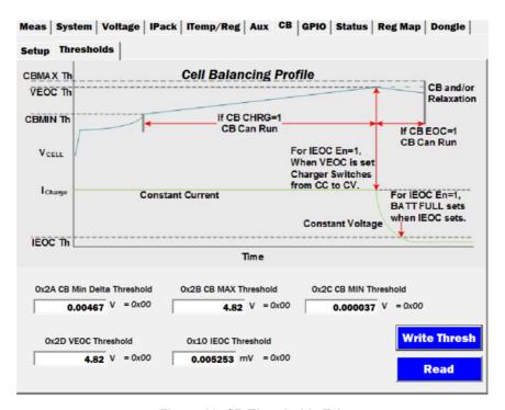
Figure 83. CB Thresholds Tab
