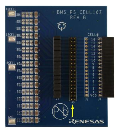
Figure 8. Resistor Ladder Board
