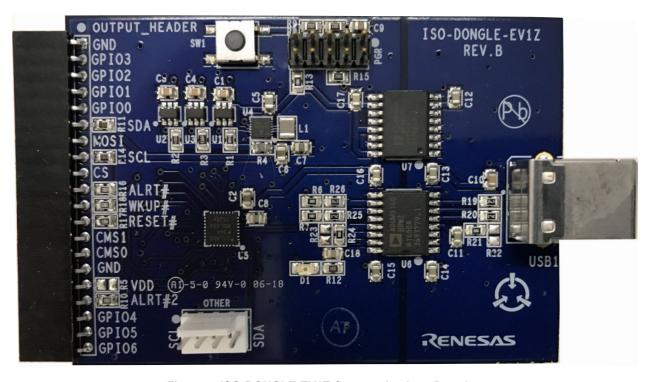
Figure 7. ISO-DONGLE-EV1Z Communications Dongle
