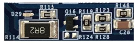
Figure 4. VC1 External Cell Balancing Circuitry
