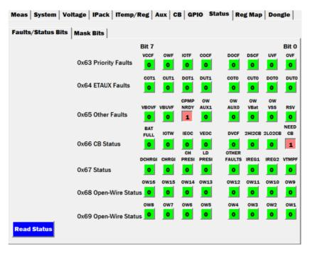
Figure 85. Faults/Status Bits Tab
