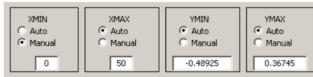
With **Auto** selected, the last 50 measurements are displayed as data collection runs. This produces a horizontal scrolling of the data.
