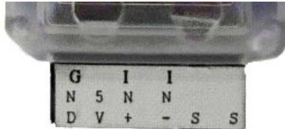
Figure 4. Sensor Connector
