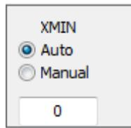
To see the history of the sensor reading from the beginning, pin the X axis to 0 by clicking **Manual** in the XMIN box and entering 0 in the selection window.
