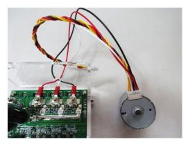
Step 5: Turn on the regulated power supply and confirm that the LED lights up.
