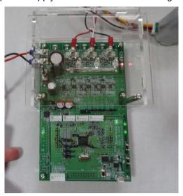
Step 6: Confirm that pressing SW1 drives the PMSM and pressing SW2 stops the PMSM.
